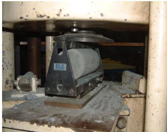
(c) Cylinder test for indirect tensile strength
