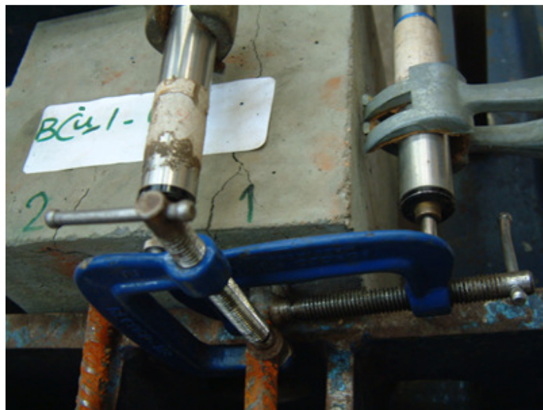
Figure 4.16: Failure mode with C` bar reinforcement
