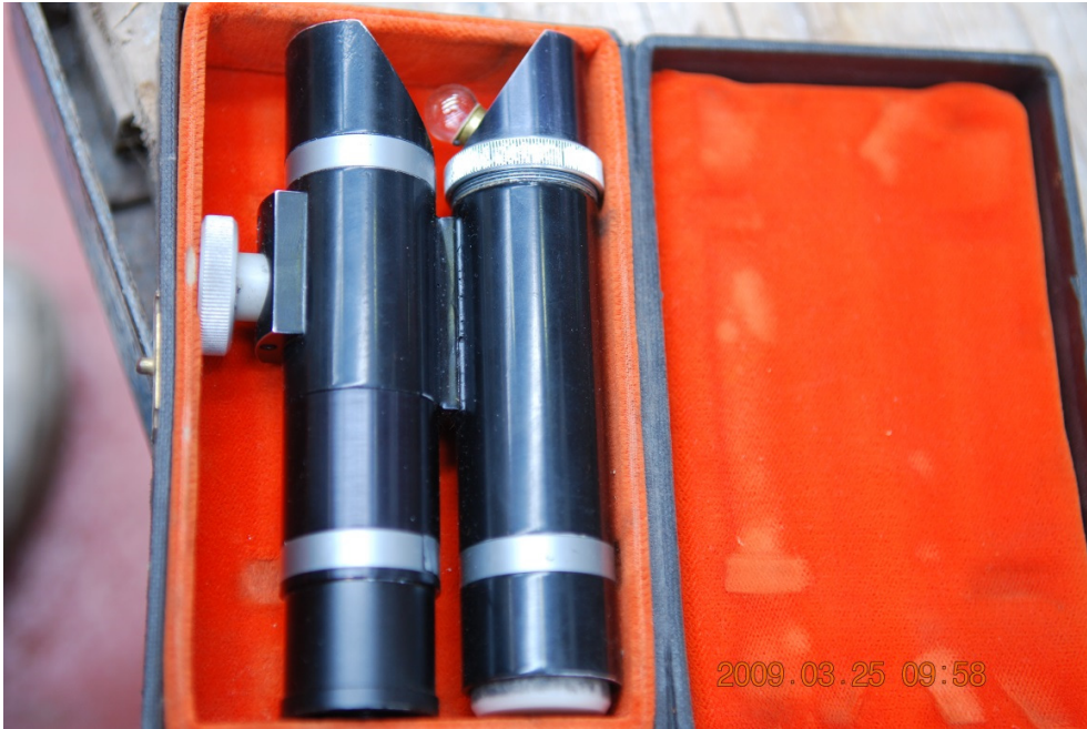
Figure 6.3: Crack comparator for measuring cracks widths during tests
