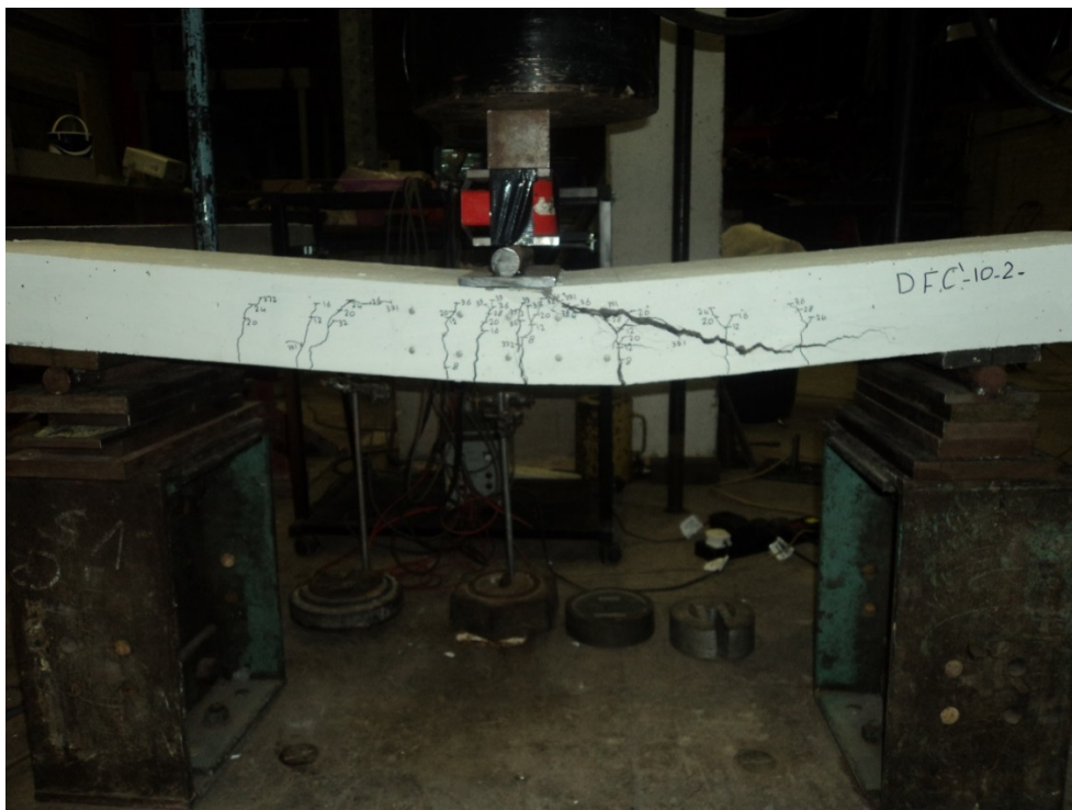
Figure 6.33: Ductility test failure mode for DFC`-10-2
