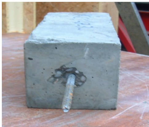
Figure 4.24: Fractured bar after pull-out test with 350 mm embedment length
