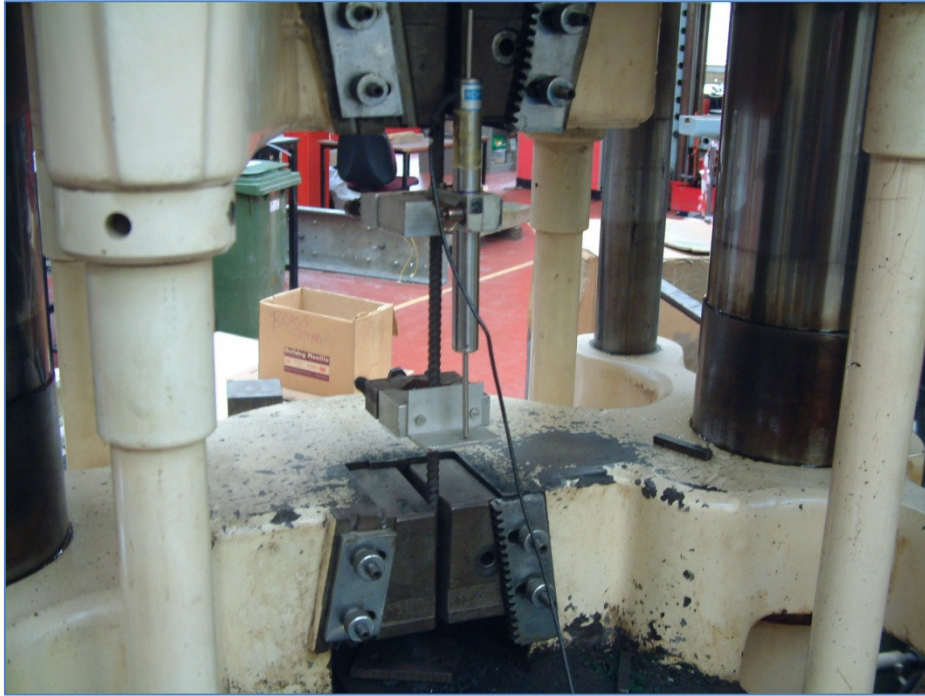
Figure 3.1: Denison machine used for steel bars tensile test
