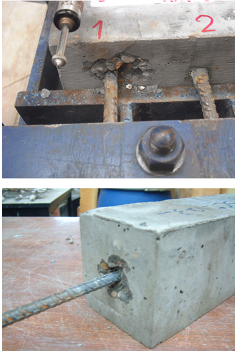
Figure 4.28: Failure modes for 20 & 40 mm concrete cover respectively pictures
