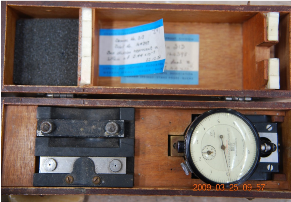
Figure 6.2: 50 mm length Demec gauge for measuring concrete strain
