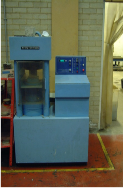
(a) Cube test for compressive strength
