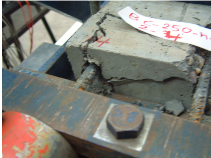
Figure 4.12: Splitting failure mode of concrete block with no shear link reinforcement
