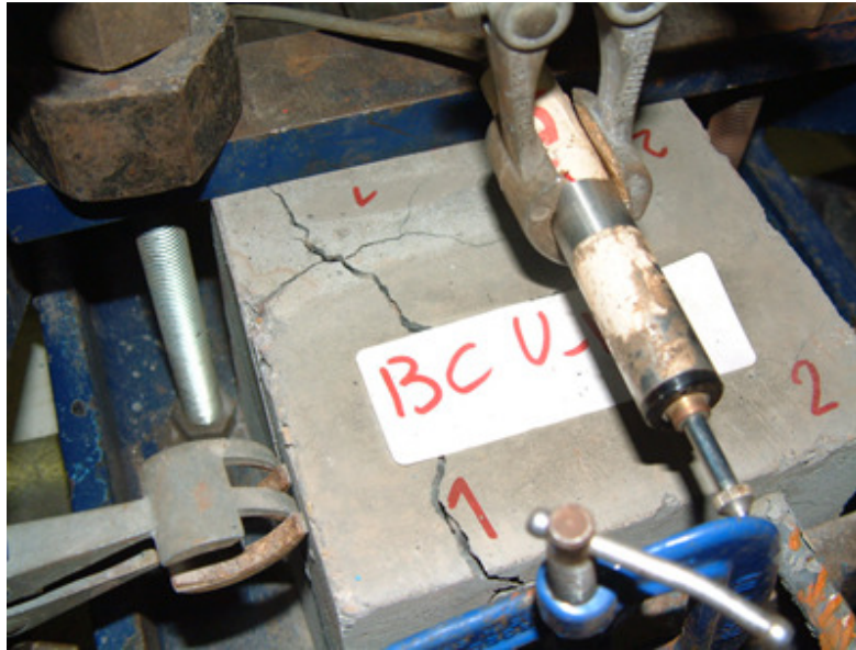
Figure 4.17: Failure mode with C bar reinforcement
