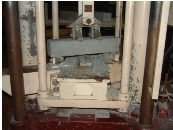
(b) Prism test for modulus of rupture
