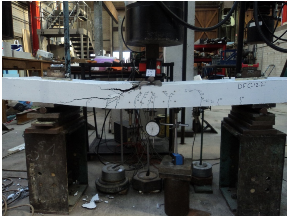
Figure 6.34: Ductility test failure mode for DFC`-12-2
