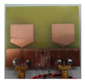
Fig. 3.2.8. Photograph of the fabricated prototype of the structure with the UWB antennas and one slit-patch structure.
