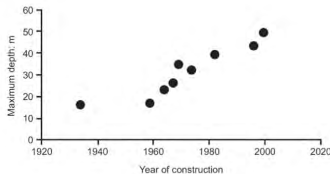
Figure 2-15: Evolution of the depth of Tokyo metro lines (Bobilev, 2009a)
