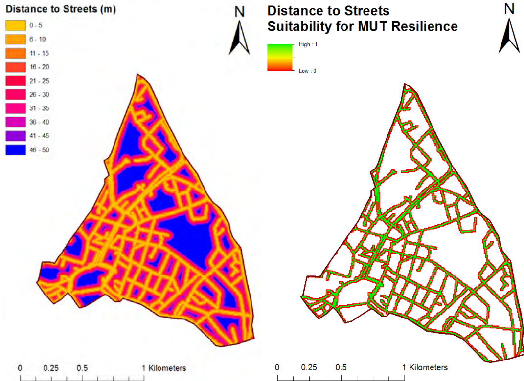
Source map and standardised/ reclassified map for the factor 'Distance to streets'
