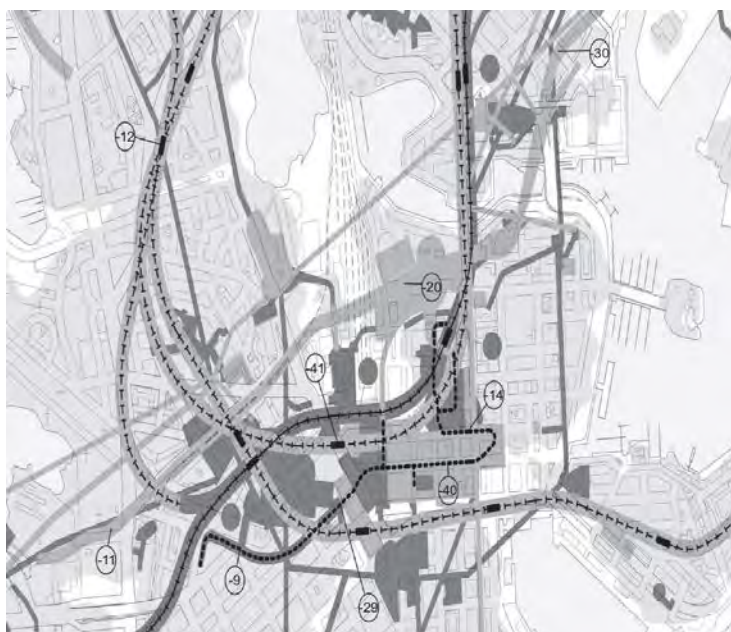
Figure 2-23: City of Helsinki underground space master plan. Circled figures indicate approximate floor elevations. Existing vital access links to underground technical maintenance spaces/tunnels are shown on the map with triangles. Grey = planned underground spaces and tunnels; dark grey = existing underground spaces and tunnels; light grey = rock resources reserved for the construction of as yet unnamed underground facilities; lightest grey = rock surface less than 10 m below ground surface (Sterling et al., 2012)
