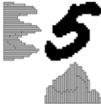
Figure 2.2: Horizontal and vertical projection histograms [TJT95]
