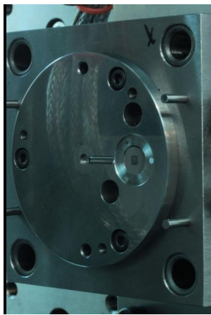
(a) Mould assembly
