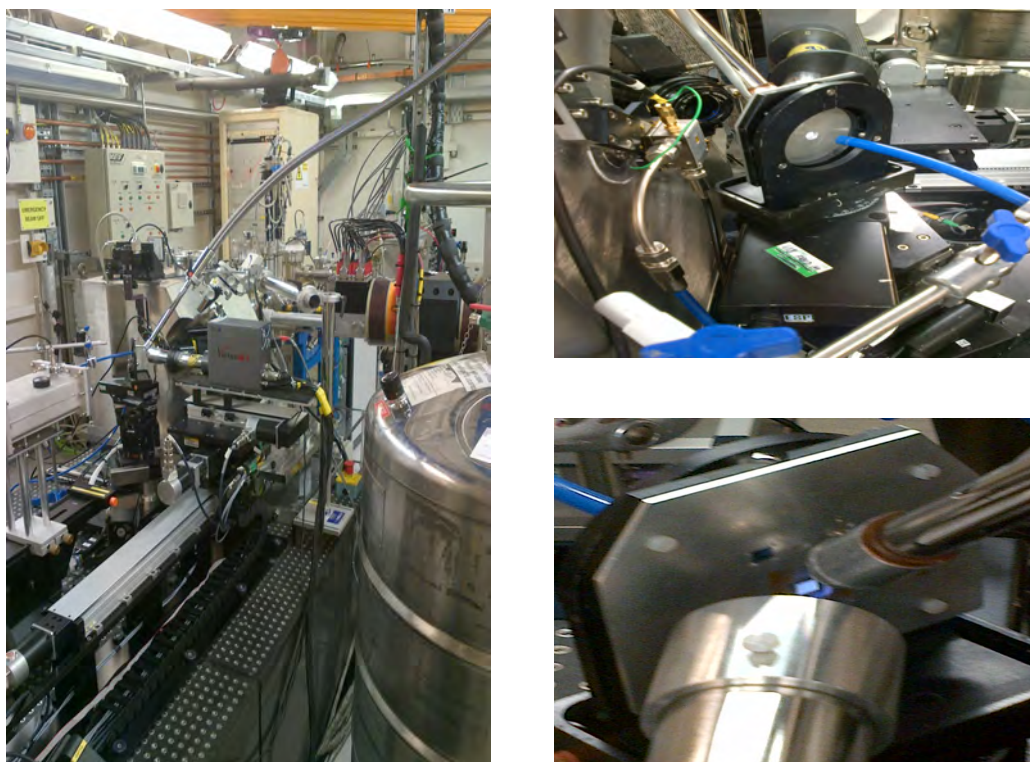
Figure 3.16: Images of experimental set up at I18 beamline. Left - view of experimental hutch, facing towards the beamline. Right - Rear (top) and forward facing (bottom) views of sample in situ . The blue pipe blows cooled nitrogen to the rear of the sample, the thinner outlet in the bottom right image is a helium cryojet - both of these are to keep the sample cold. The large apparatus seen in the bottom right image is the detector, held at 45° to the sample.
