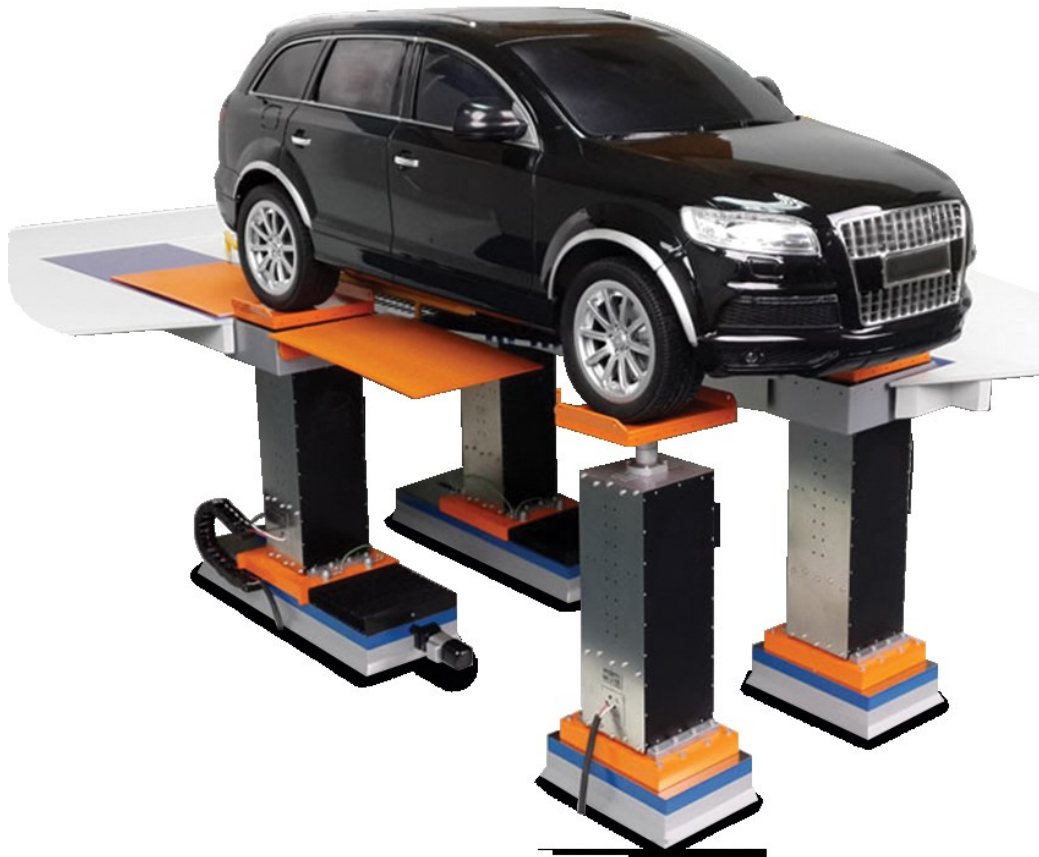
Figure 2.1: A Tyre-Coupled RTS courtesy of MTS Systems Corporation
