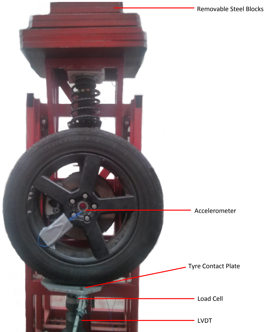
Figure 3.1: Quarter Vehicle and Suspension Unit
