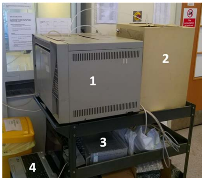
Figure 31: Exposure vessel assembly. 1: GC oven; 2: heater/bubbler; 3: MFC controller and MFCs; 4: Computer controlling MFCs and gas flows.
