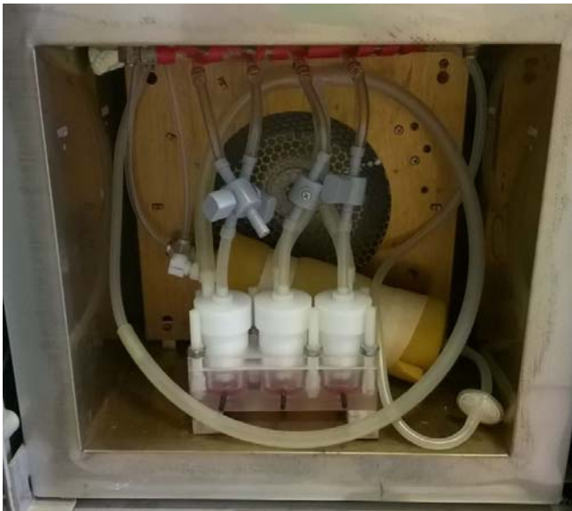
Figure 30: Assembled exposure vessel in working order, hosted inside the GC oven.
