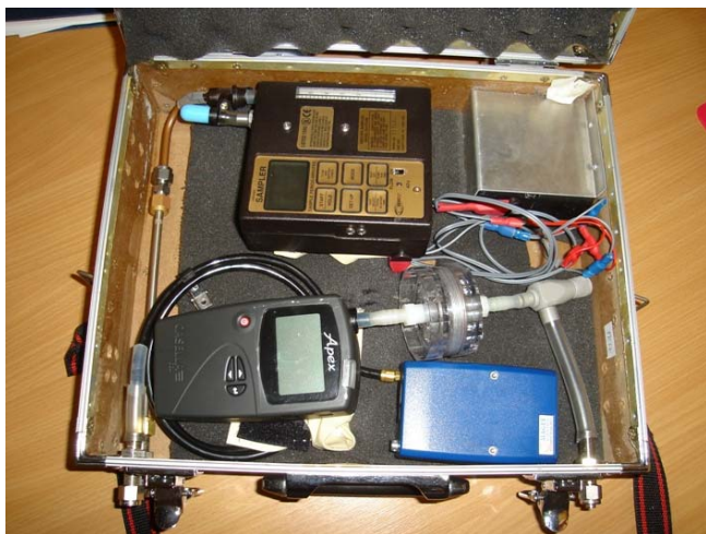
Figure 26: Sampling briefcase, containing a VOC pump (top), connected to a sorbent tube and a PAH pump (bottom, black) connected to a quartz filter and the micro aethalometer (bottom, blue).
