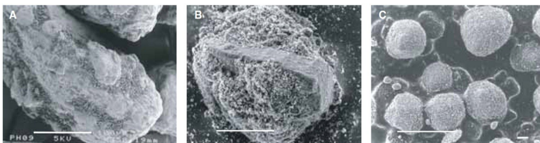
Fig. 2.3. SEM pictures of three types of formulation: a) an adhesive mixture, b) a nucleus agglomerate and c) a spherical pellet (Frijlink and De Boer, 2004).
