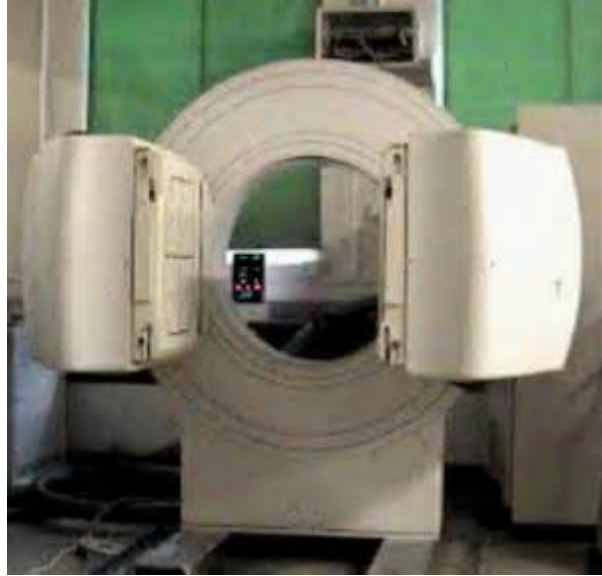
Figure 3.1: The modified dual-headed positron camera used to acquire PEPT data.
