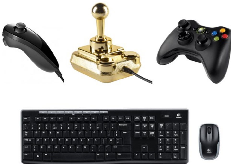
Figure 6.1 Four Input Devices Used in the Usability Studies. (Upper left: Nunchuk thumb controller; Upper mid: Joystick; Upper right: Xbox wireless controller; Bottom: Keyboard and mouse)
