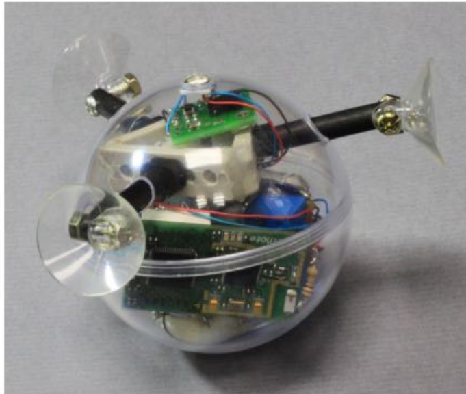
Figure 2.20 Prototype of the TriopusNet node (Lai et al., 2012).
