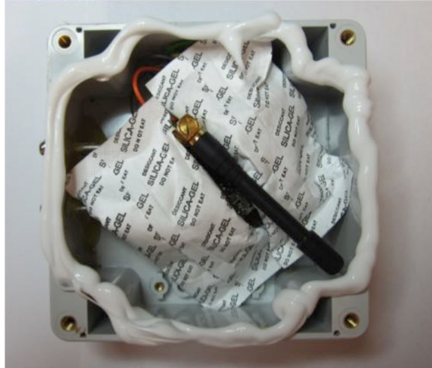
Figure 5.12 Sealing of node C
