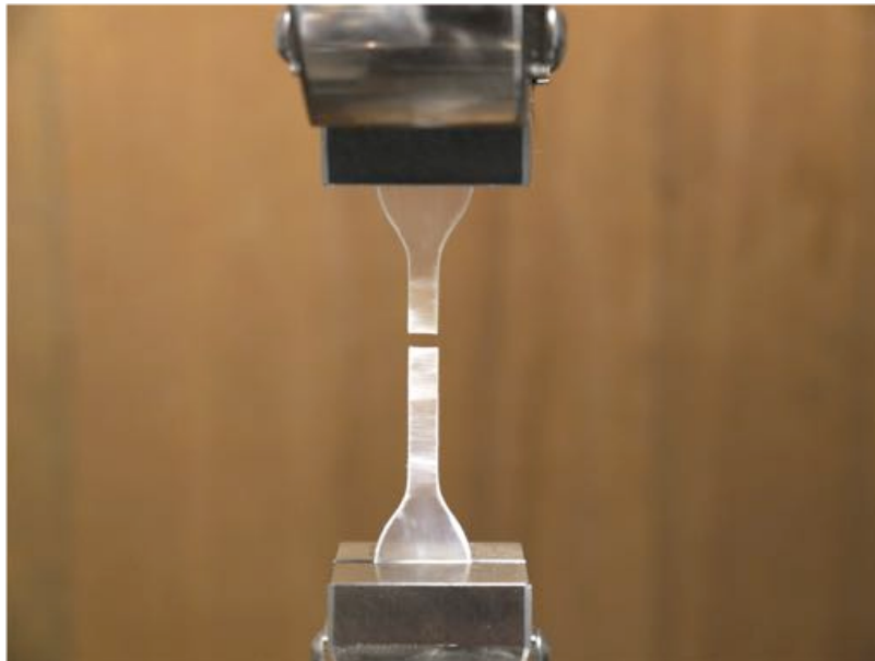
Figure 2.17. Failure of a brittle polymer sample.
