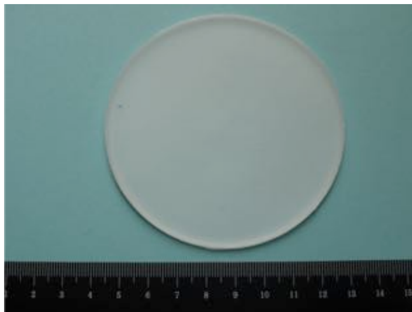
Figure 3.1. PCL 6800 solvent cast sample. A smooth, homogeneous surface finish obtained by the slow evaporation of the solvent.
