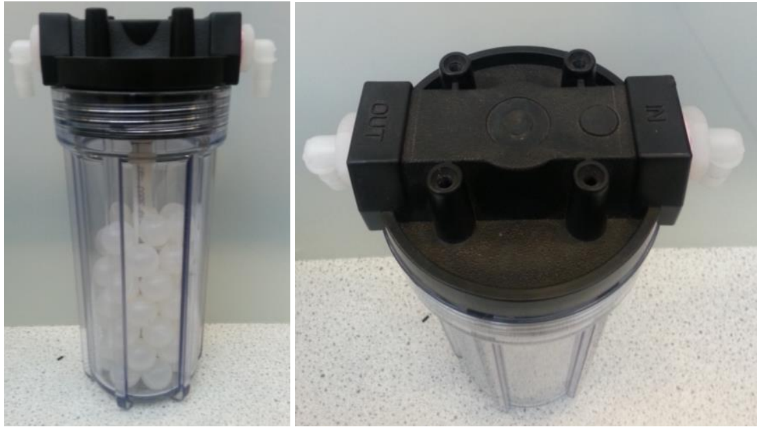
Figure 4.6: Image of commercially supplied water trap made up of Silica spheres
