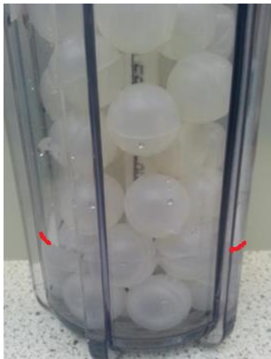
Figure 4.8: Water Trap after Engine Integration with Red Line marking Water Level
