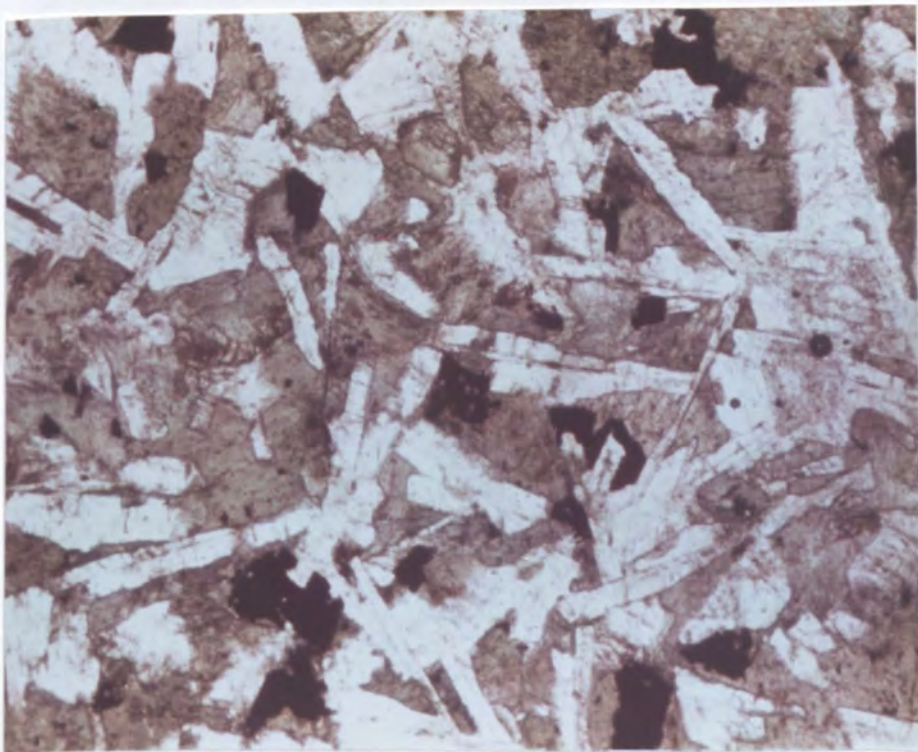
(b) Same metadolerite in plane polarized light. X134 ppl. X12.5
