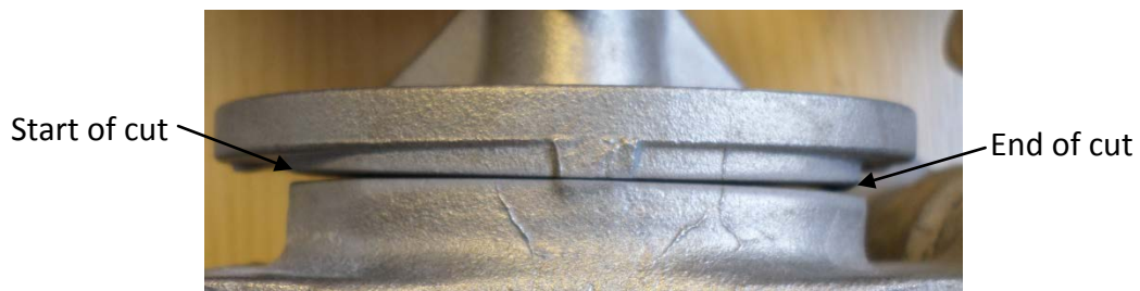
Figure 4- 29: Kerf width increase at the start and end of tibial cut
