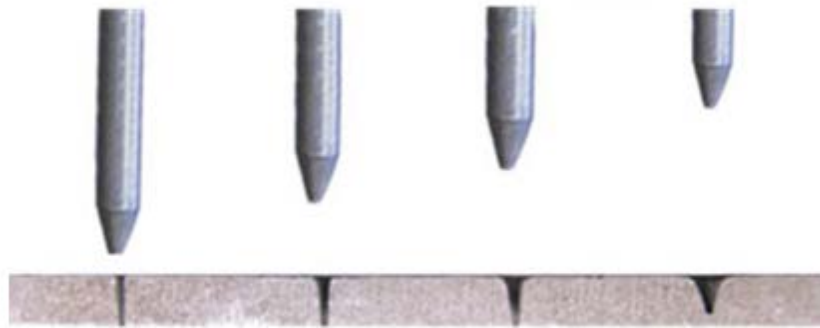
Figure 5- 1: Effect of increasing standoff distance (WARDJet, 2013a)
