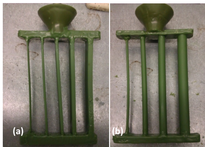
Figure 3- 4: Improved wax tree designs: (a) flat bars 2, 4, 6, 8 and 10 mm thick (b) cylinders 5, 10, 15 and 20 mm diameter
