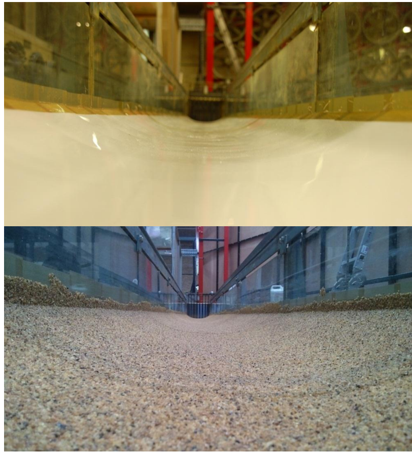
Figure 27. Downstream view of the channel without water. Above on smooth surface (PVC). Below on rough surface (glue sand).
