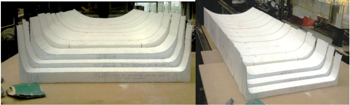
Figure 45. The material used in the transition was polystyrene. Several transversal panels were cut, and later sanded down.
