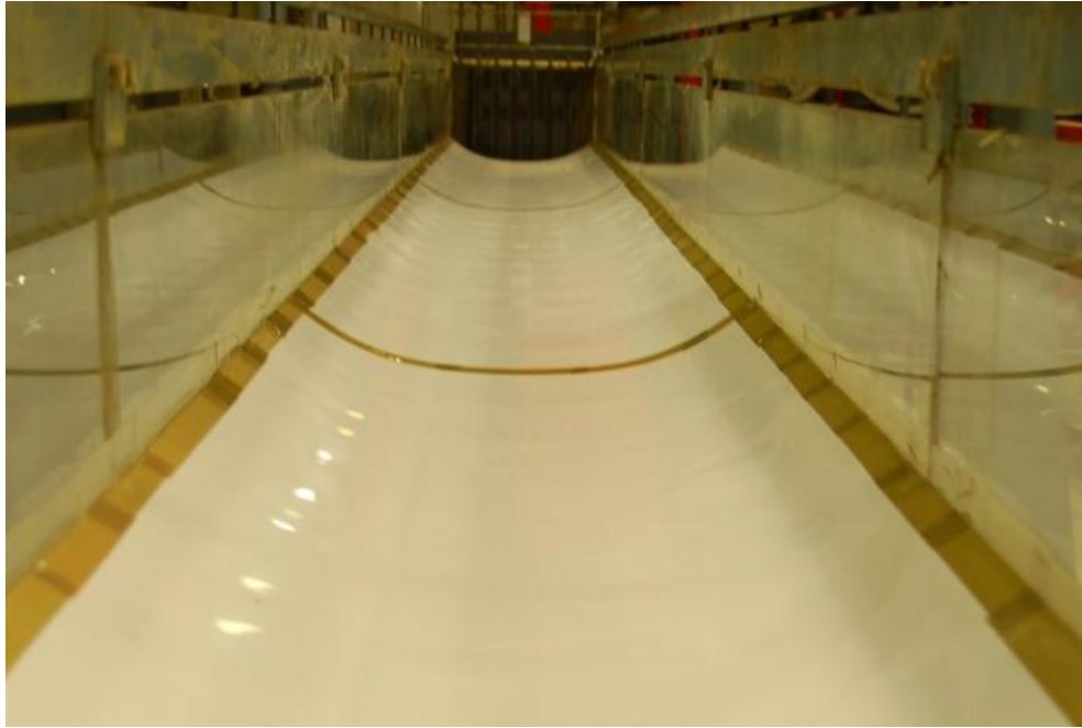
Figure 36. In order to avoid leakage, brown tape was placed between the boundaries.
