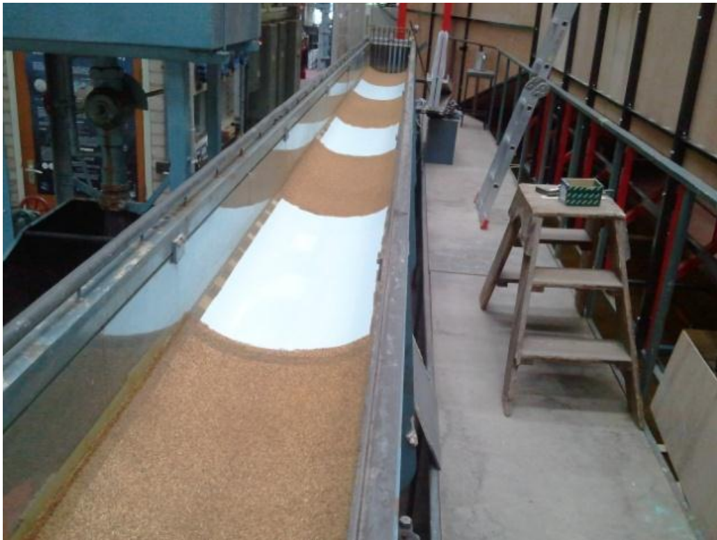
Figure 37. Glue sand ( d_{50}=1.46\text{mm} ) was applied by segments.
