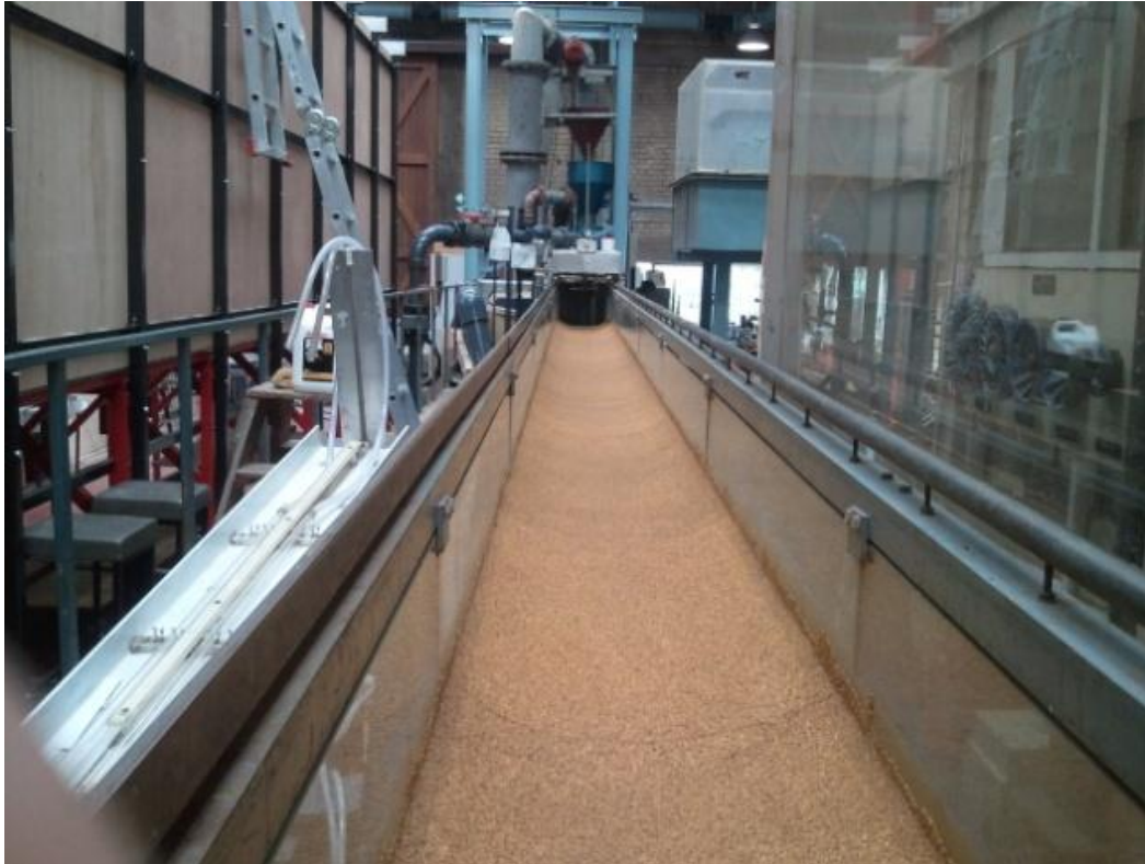
Figure 39. The full length of the channel with glue sand surface.
