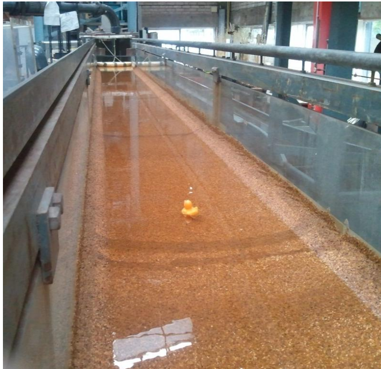
Figure 26 . Upstream view of the flume during experiments on glue sand surface. Approximated depth: h_c=3.5\text{cm} .
