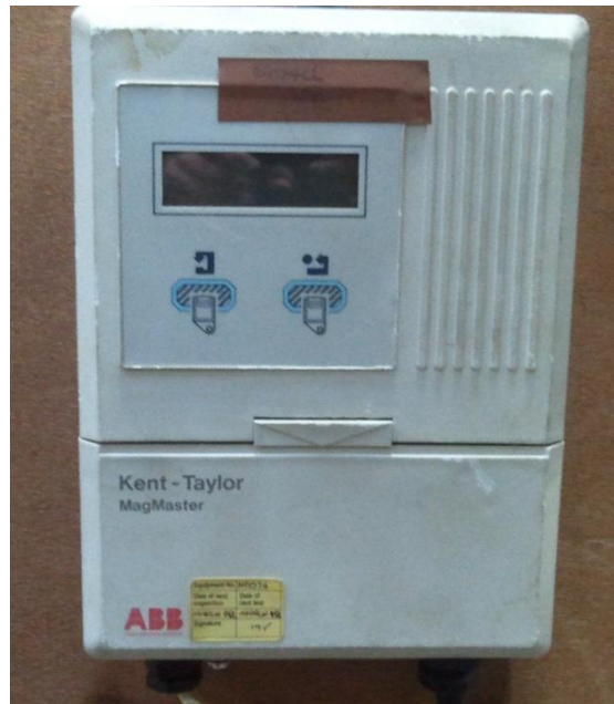
Figure 30. Electromagnetic flowmeter used during the experiments: ABB Kent-Taylor MagMaster.
