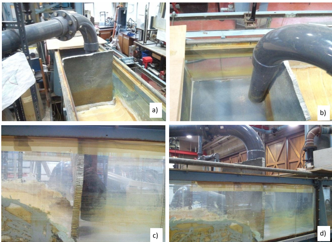
Figure 29. View of the delivery pipe at the entrance of the flume. Four perspective are provided: (a) view from downstream; (b) aerial view; (c) profile view, pipe delivering and transition; and (d) downstream profile view.
