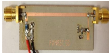
Figure 4.11-Photographs of the fabricated STS MN in case 1 (switch in the middle of the stub)
