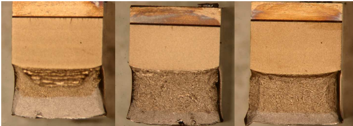
Figure 5.36: Fracture surface of respective O2 weld samples FT004 and FT008 (Hoop) and FT005 (Radial) at 400°C
