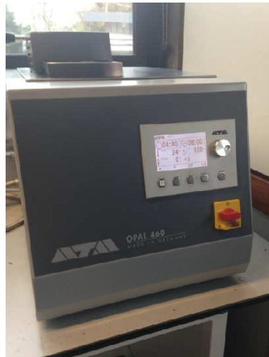
Figure 4.5: Opal 460 Mounting Press
