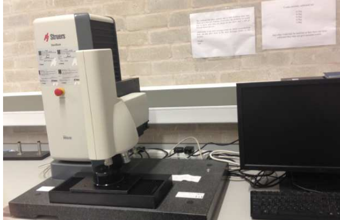
Figure 4.11: Struers automatic hardness testing machine
