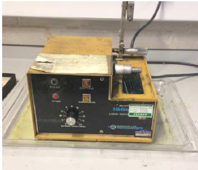
Figure 4.13: Buehler Isomet – slow speed saw with a silicon cutting blade
