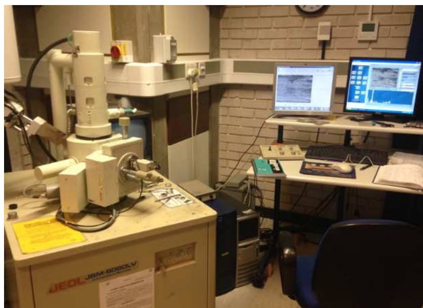
Figure 4.9: Jeol 6060 with Oxford Inca EDS
