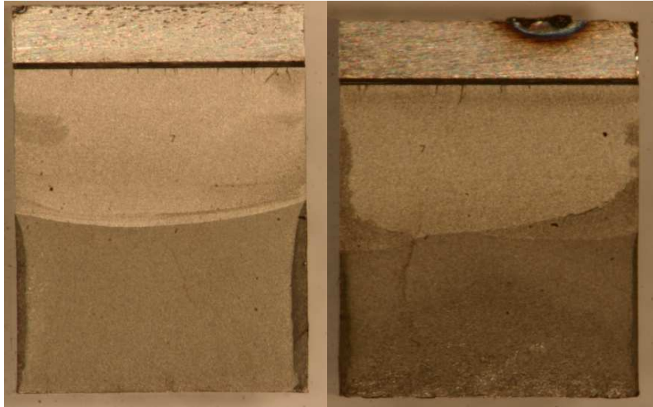
Figure 5.35: Fracture surface of respective O2 weld samples FT003 (Hoop) and FT006 (Radial) at RT
