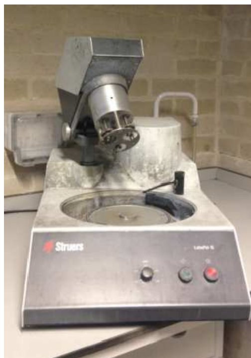
Figure 4.6: Struers Labopol-5 automatic polishing machine
