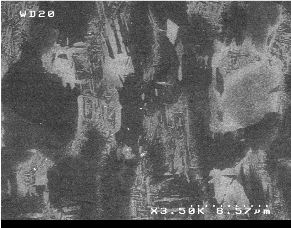
Figure 5.17: SEM image of the HAZ observed at X3500 magnification showing the transformed \beta phase and coarse acicular \alpha
