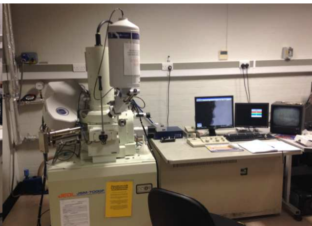
Figure 4.8: Jeol 7000F with Oxford Inca EDS, Wave WDS and Crystal EBSD
