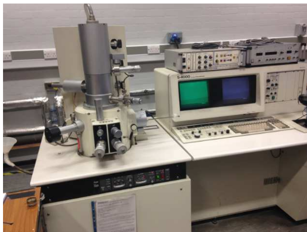
Figure 4.7: S4000 field emission gun (FEG) electron microscope
