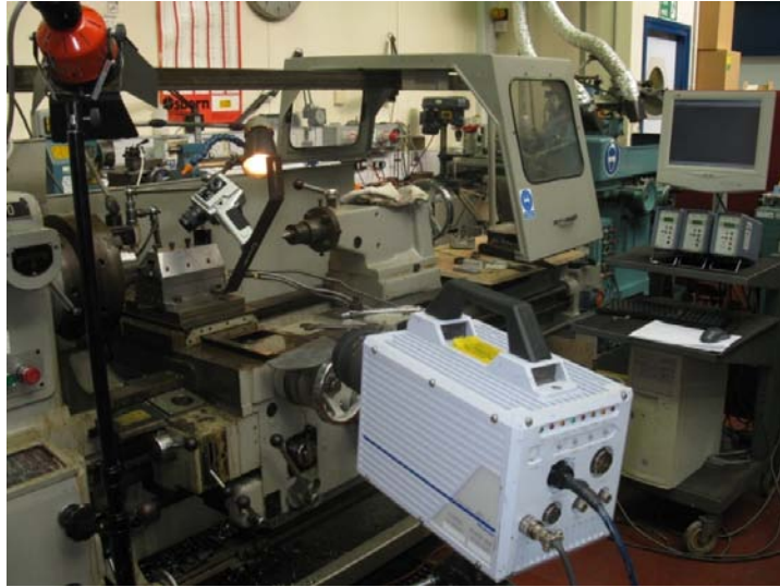
Figure 49. Complete setup prepared previous to the machining trials on Inconel 718.
