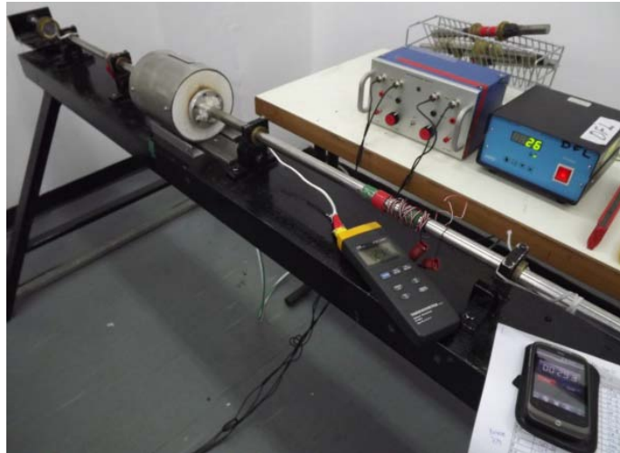
Figure 43. Thermal calibration setup.
