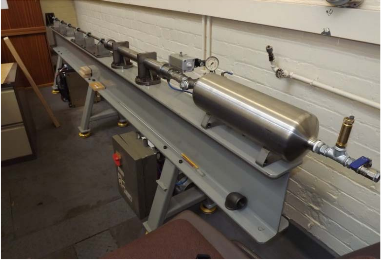
Figure AI.7. SHPB apparatus assembly.
