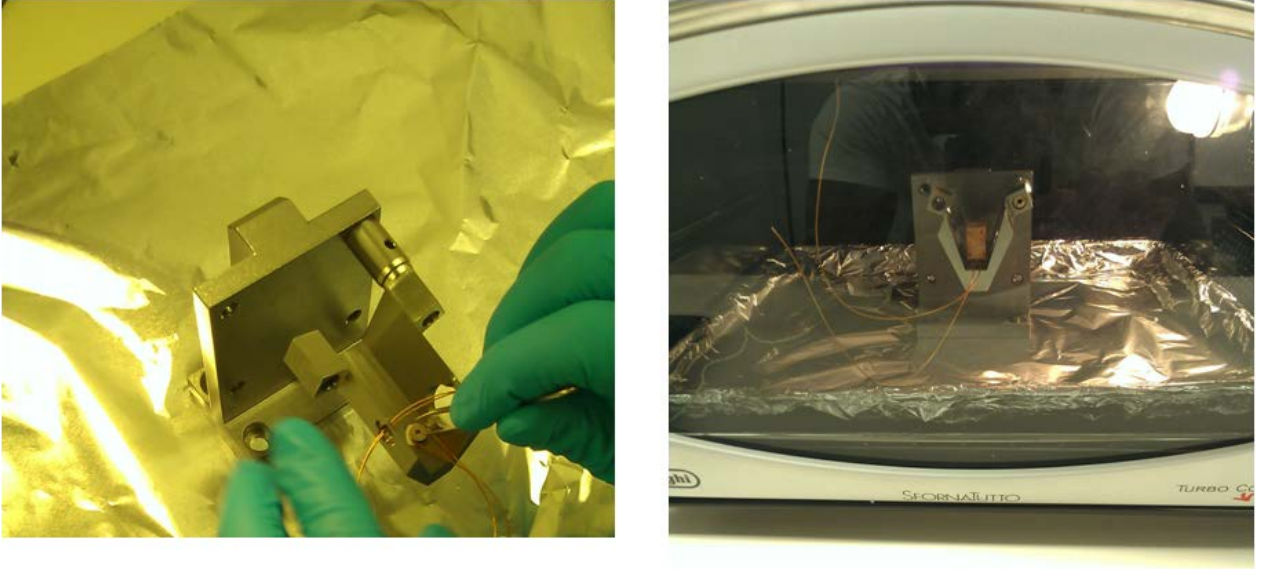
Figure 6.5: Cavity mirror gluing and heat curing procedure in portable oven.
