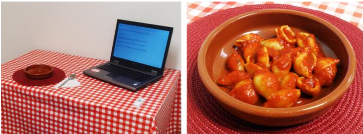
Figure 2.1 Left panel shows the UEM setup, featuring the laptop computer connected covertly to the balance underneath the red table mat with the dish for pasta placed on top. Right panel shows a standard 200g serving of the tomato-based pasta on the UEM setup.
