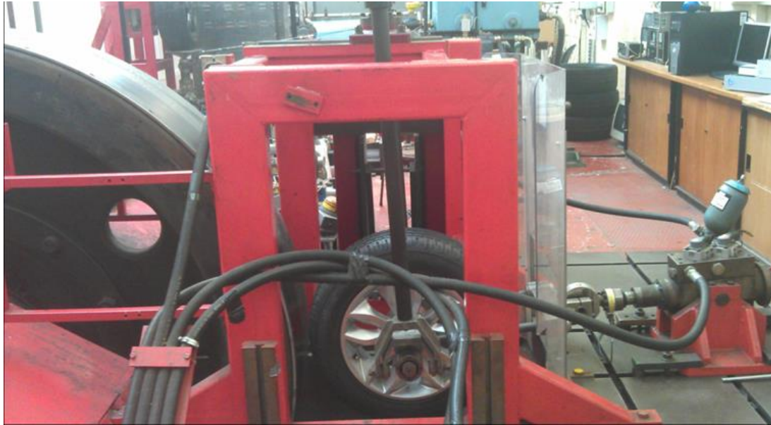
Figure 4.10 Tri-axial electro-hydraulic test rig
