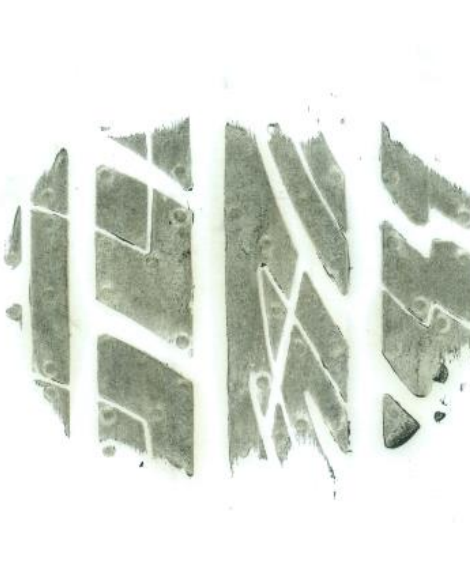
Figure 4.27 Footprint for 2000N vertical load, 200kPa inflation pressure
