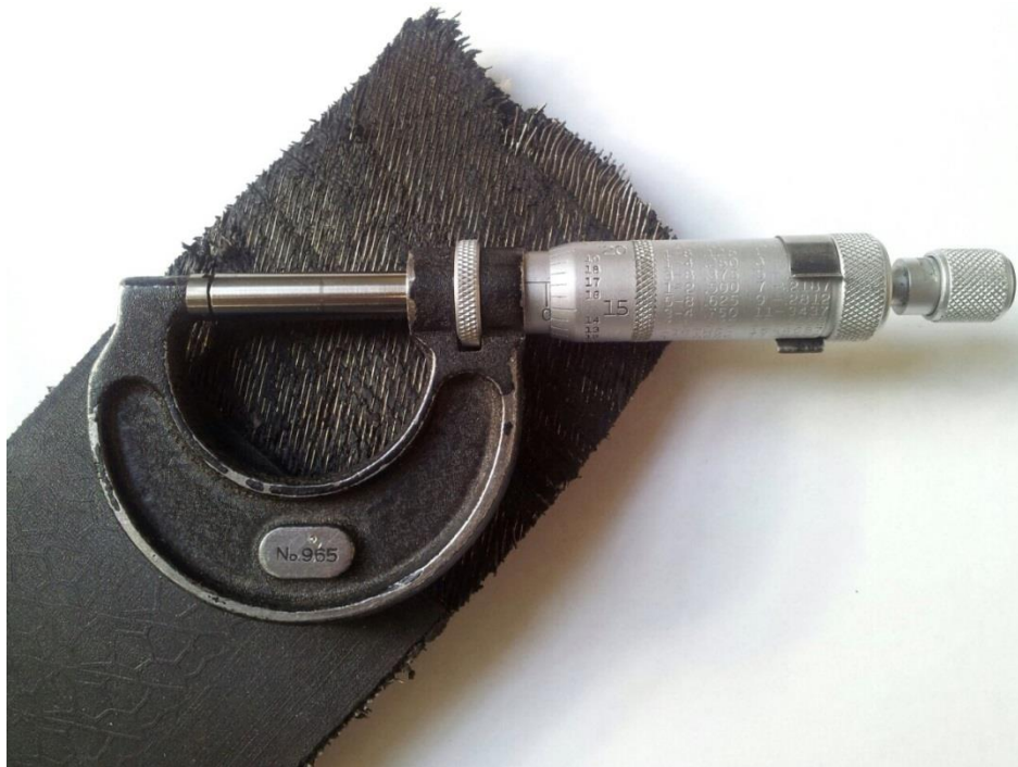
Figure 3.8 Area measurement for cross section of steel belt
