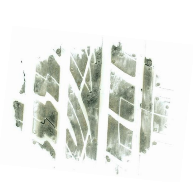
Figure 4.28 Footprint for 3000N vertical load, 200kPa inflation pressure
