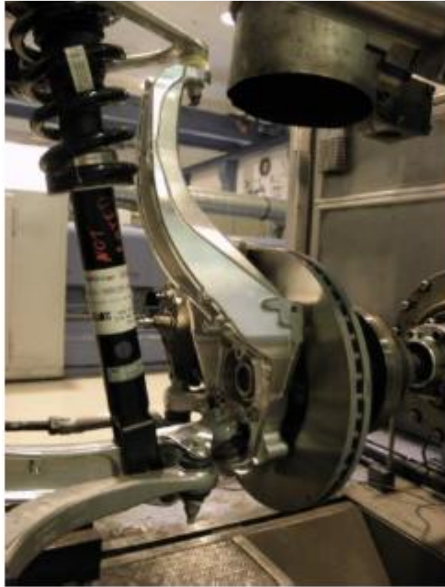
Figure 2, Brake corner unit mounted on the dynamometer
