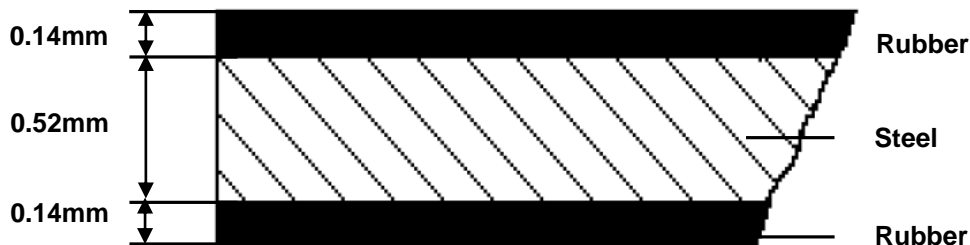
Figure 49, Schematic of three layer shim design
