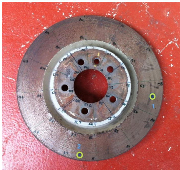
Figure 30, Brake disc - hammer test markings
