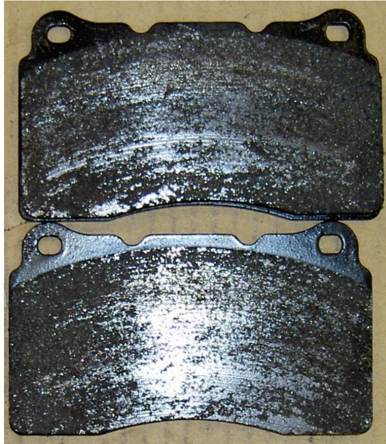
Figure 84, Post-test brake pads – 2 partitions
