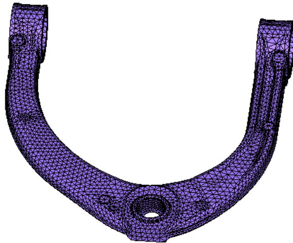
Figure 22, CAE model - upper control arm
