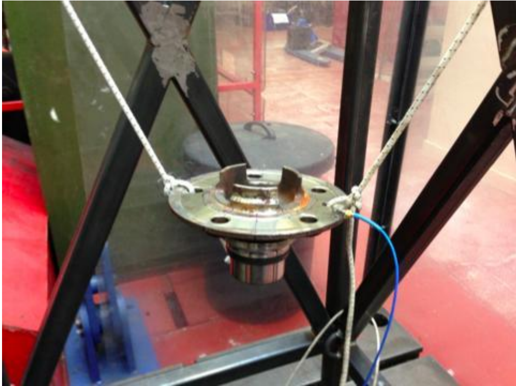
Figure 10, Brake hub hammer test (UOB)
