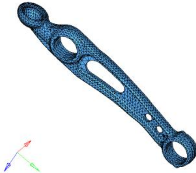
Figure 23, CAE model - lateral control arm
