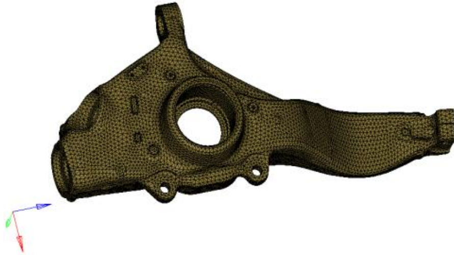
Figure 20, CAE model - brake knuckle
