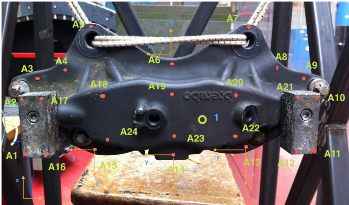
Figure 33, Brake caliper, hammer test markings (side)
