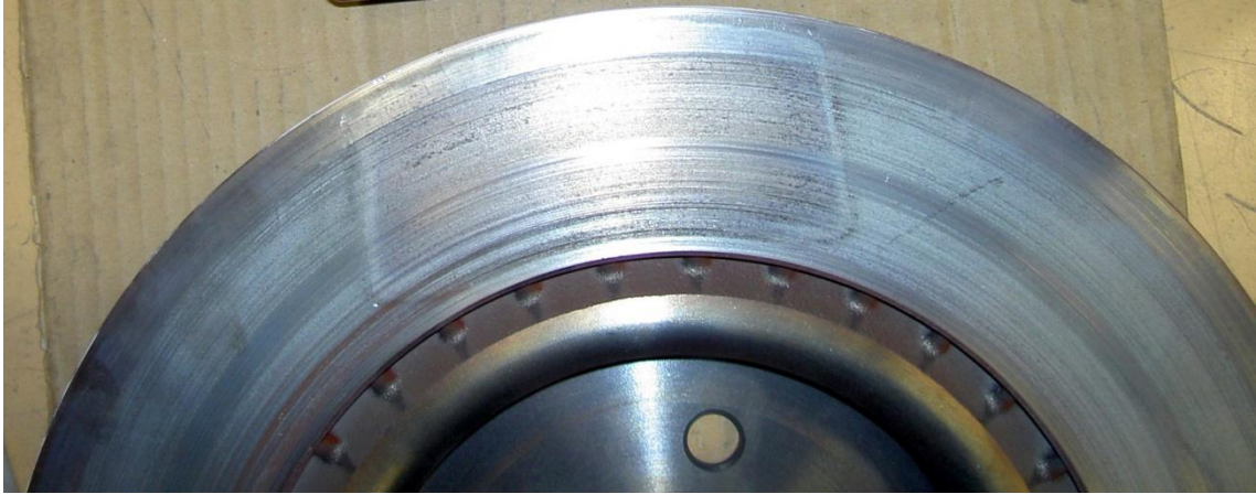
Figure 85, Post-test brake disc
