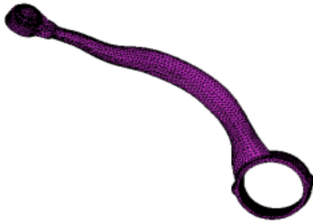
Figure 21, CAE model - front tension arm
