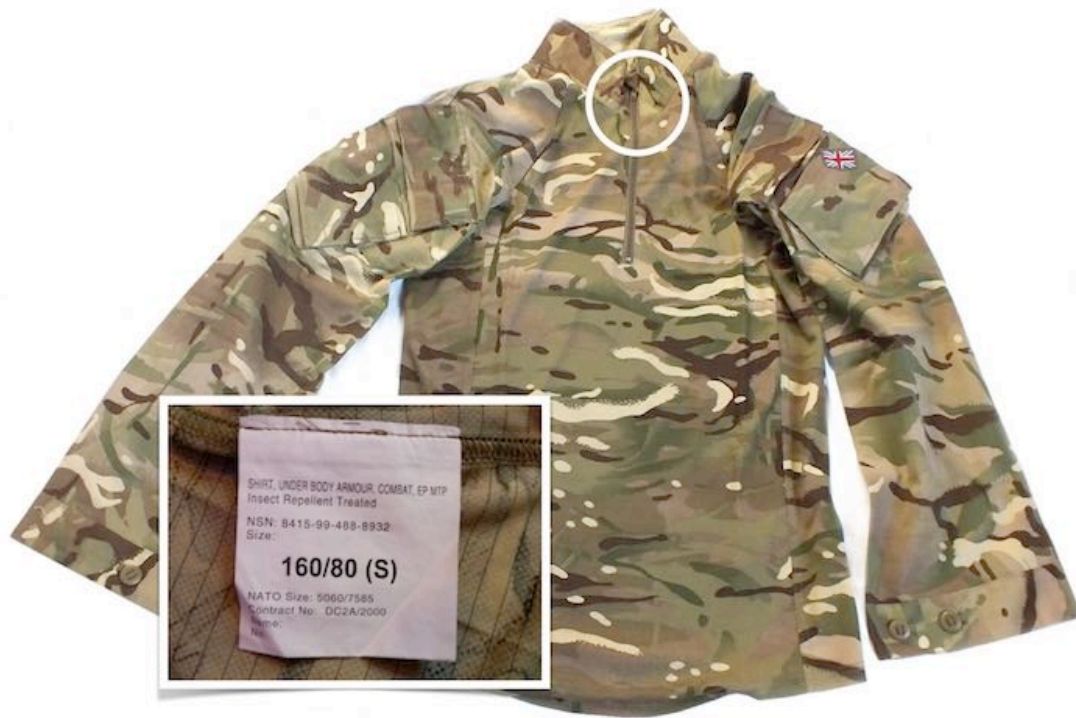
Figure 92: The EP- UBACS issued to all UK armed forces since November 2013 incorporates UHMWPE felt in the neck collar (box insert). Note Modified Terrain Pattern is used throughout and a slip of material covers the zip at the top (circled).
