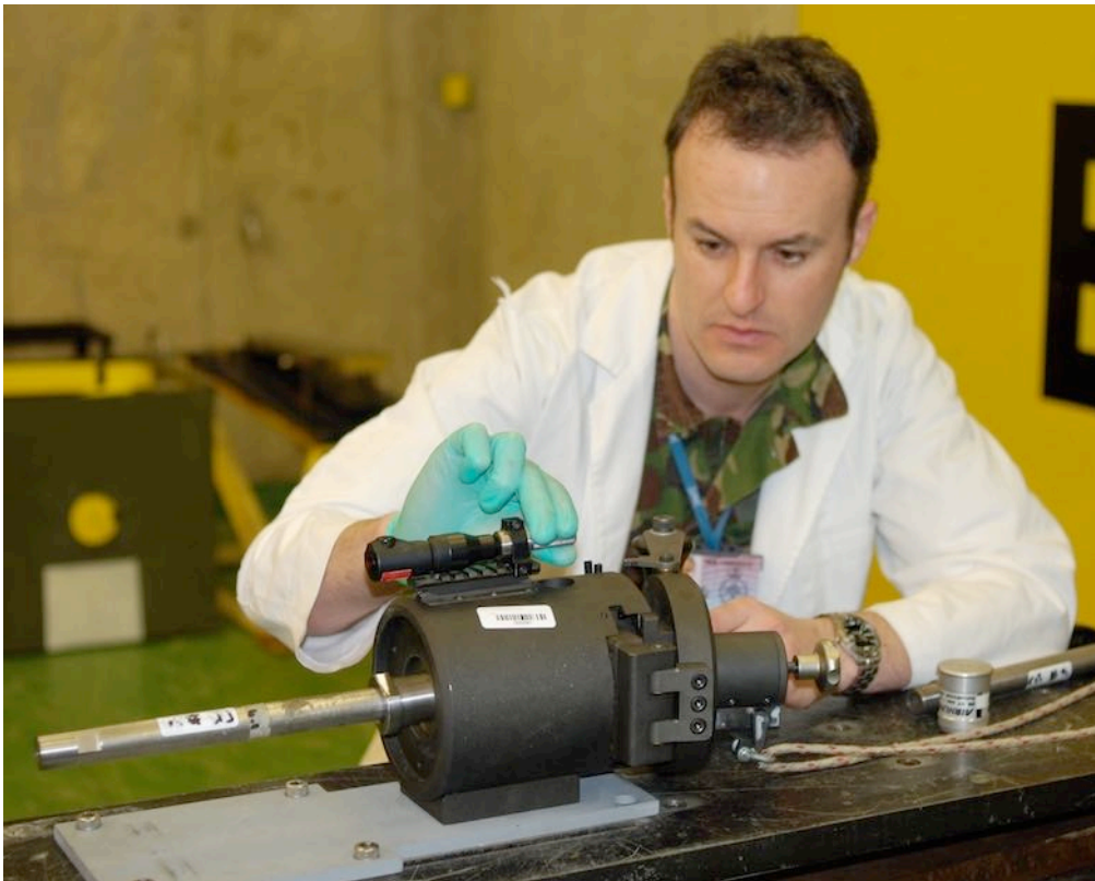
Figure 13: The author assisting in the testing of a number of ballistic protective materials to ascertain V_{50} velocities using a 1.10g FSP fired from a gas gun.
