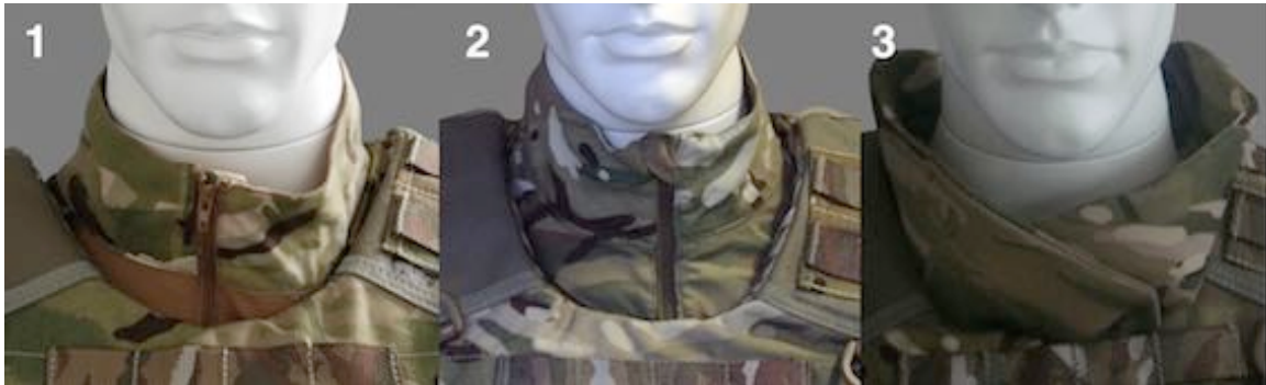
Figure 35: Modified UBACS neck collar prototypes 1-3 fitted on an anatomical mannequin.
