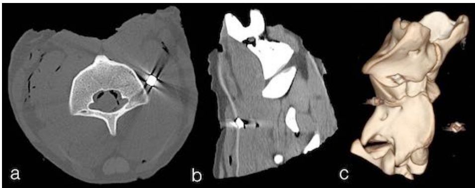
Figure 42: Computed Tomography scans taken after testing of cylindrical FSPs into a goat neck. The bony anatomy is potentially representative of a human but the vasculature is not.
