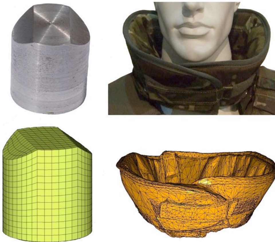
Figure 40: Meshed images of a chisel-nosed cylindrical fragment simulating projectile and the Mark 4a OSPREY half neck collar.
