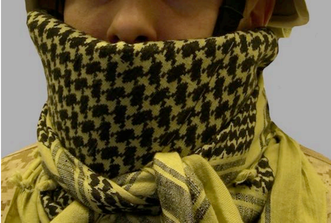
Figure 12: A ballistic scarf in which the standard cotton shemagh is reinforced with a central square of a para- aramid ballistic fibre.
