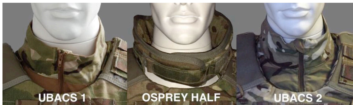
Figure 69: The modified UBACS prototype 1 has protective material in the collar alone, but there is still a gap between the OSPREY half collar and vest that is not covered by the OSPREY half collar. This gap is prevented by an additional semi circle of material below the collar in the UBACS prototype 2.
