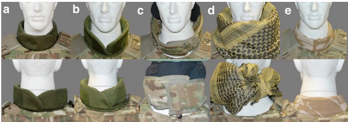
Figure 33: The five prototypes assessed in this trial compared on the same anatomical mannequin; a) Three-piece neck collar, b) Two-piece neck collar, c) Nape pad, d) Ballistic Shemagh, e) UBACS incorporating modified neck collar.
