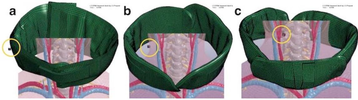
Figure 86: The OSPREY half collar (a), two-piece (b) and three-piece prototypes (c) incorporated into the FE model being run with the same 1.10g FSP (circled).
