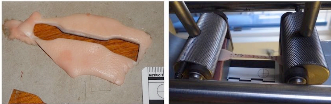
Figure 88: A sample of pig skin (left) has been placed into a device capable of generating a constant strain (right) causing distortion of the tissue measured using digital image correlation.
