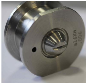
(a) Orifice ( 3.87 \text{ mm}^2 or 0.0060 \text{ in}^2 ; hereafter denoted as “orifice type 0060” or just 0060).
