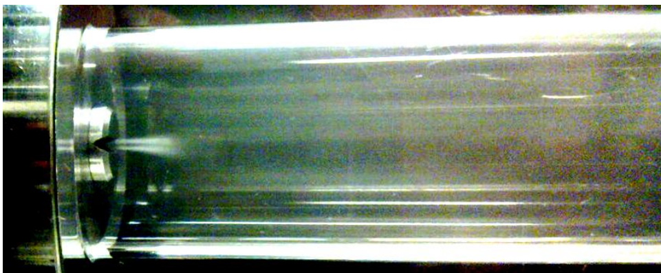
Appendix Fig 1: Photograph of Perspex Sonolator at high flow rate with twin cavitation jets originating from orifice
