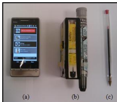
Fig. 3.5 (a) PervaLaxis 2 smartphone device; (b) AAI trainer with a three-axis Bluetooth™ accelerometer; (c) Pen size comparison.
