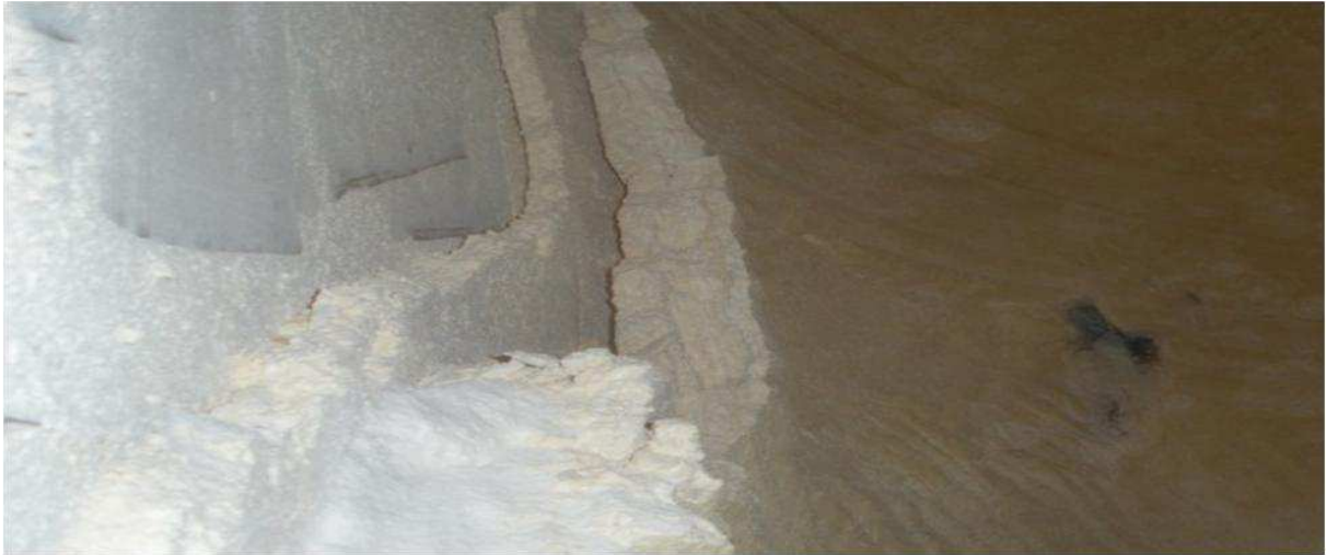
Figure 3. A transversal cut of the deposits at the wall of Scale III. It illustrates how showing a substantial thickness, deposits are homogeneously distributed and the roughness height remains constant, similar to that observed in Scale I, cases A or B.
