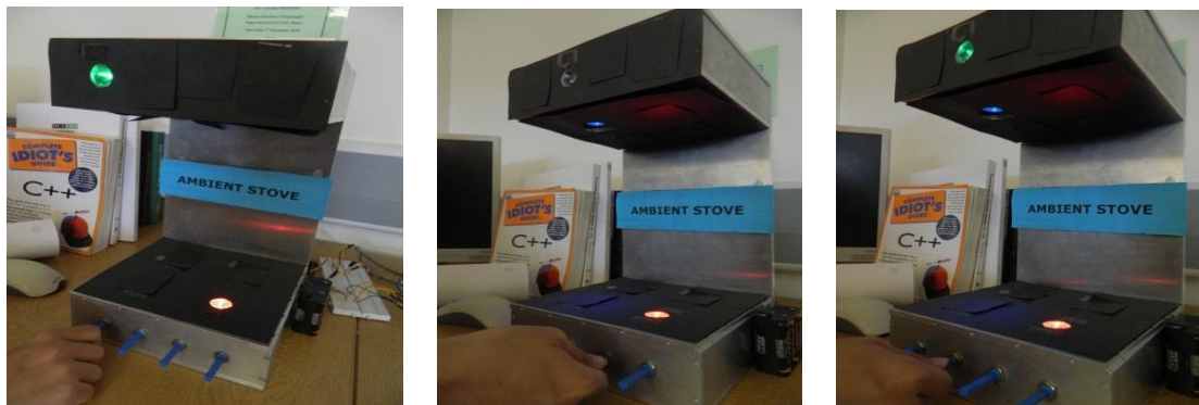
Figure 5.4 Participant responds to 2 or 3 combination of LEDs, from L to R: Red-Green, Red-Blue and Red-Green-Blue
