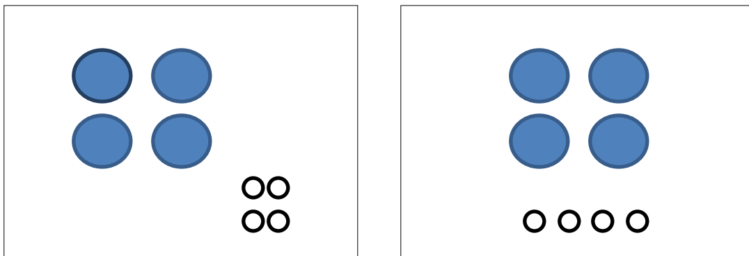
Figure 3.1 Layout of 2 x 2 control and burner with the left (L) figure is compatible arrangement control-burner and the right (R) figure is incompatible arrangement control-burner.
