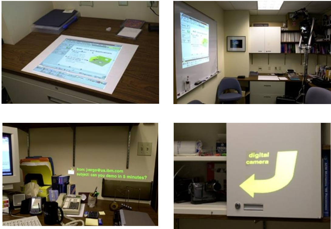
Figure 2.7 - IBM's Everywhere Display from clockwise: Interactive whiteboard, Locating equipment in an environment, Notification messages and display on desk.
