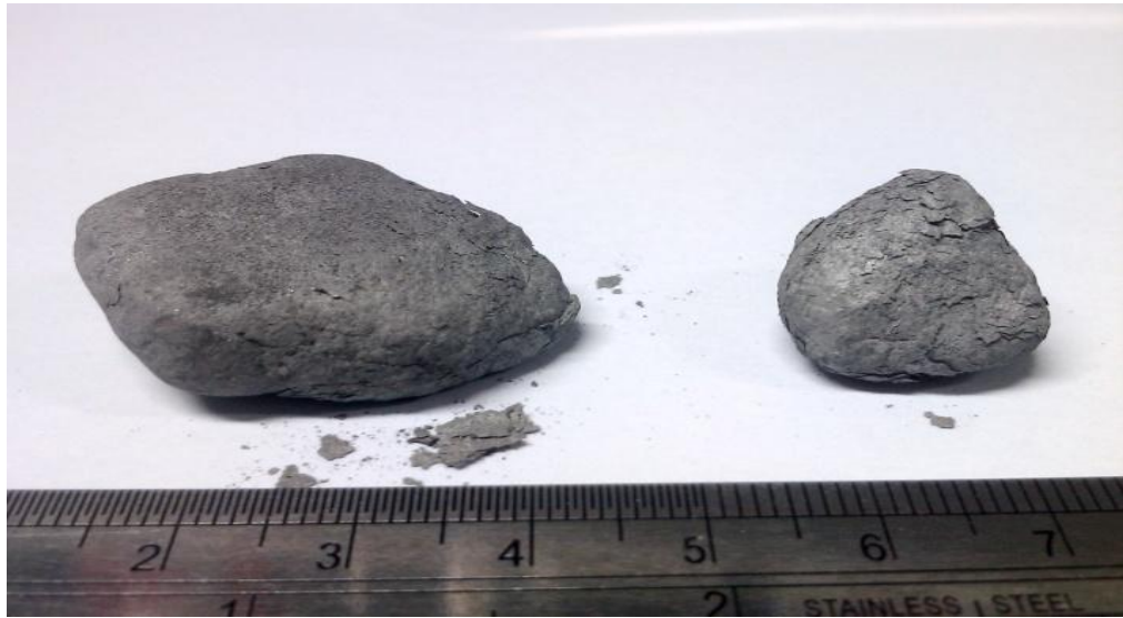
Fig.60. Two partially hydrogenated blocks which started as fractured, rectangular, uncoated sintered magnets.
