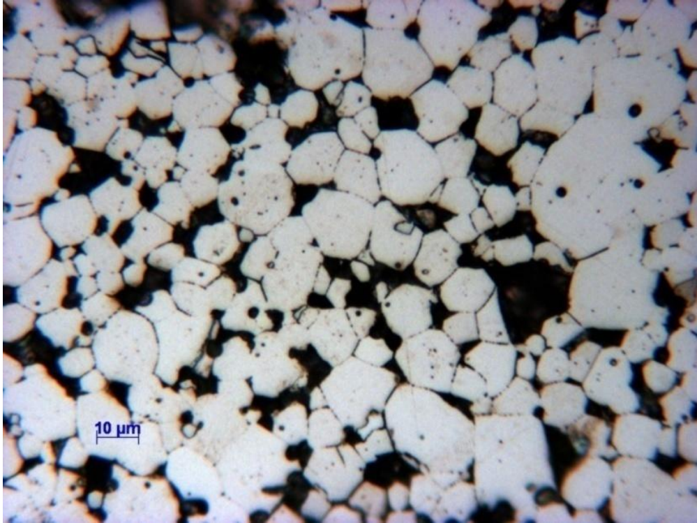
Fig.144. Powder exposed to air for 4hrs with 2at% added prior to sintering (micron marker 10μm).
