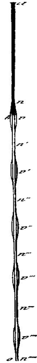
Figure 1.4: The image is taken from the Savart's original paper [77] which shows the perturbations growing on a water jet
