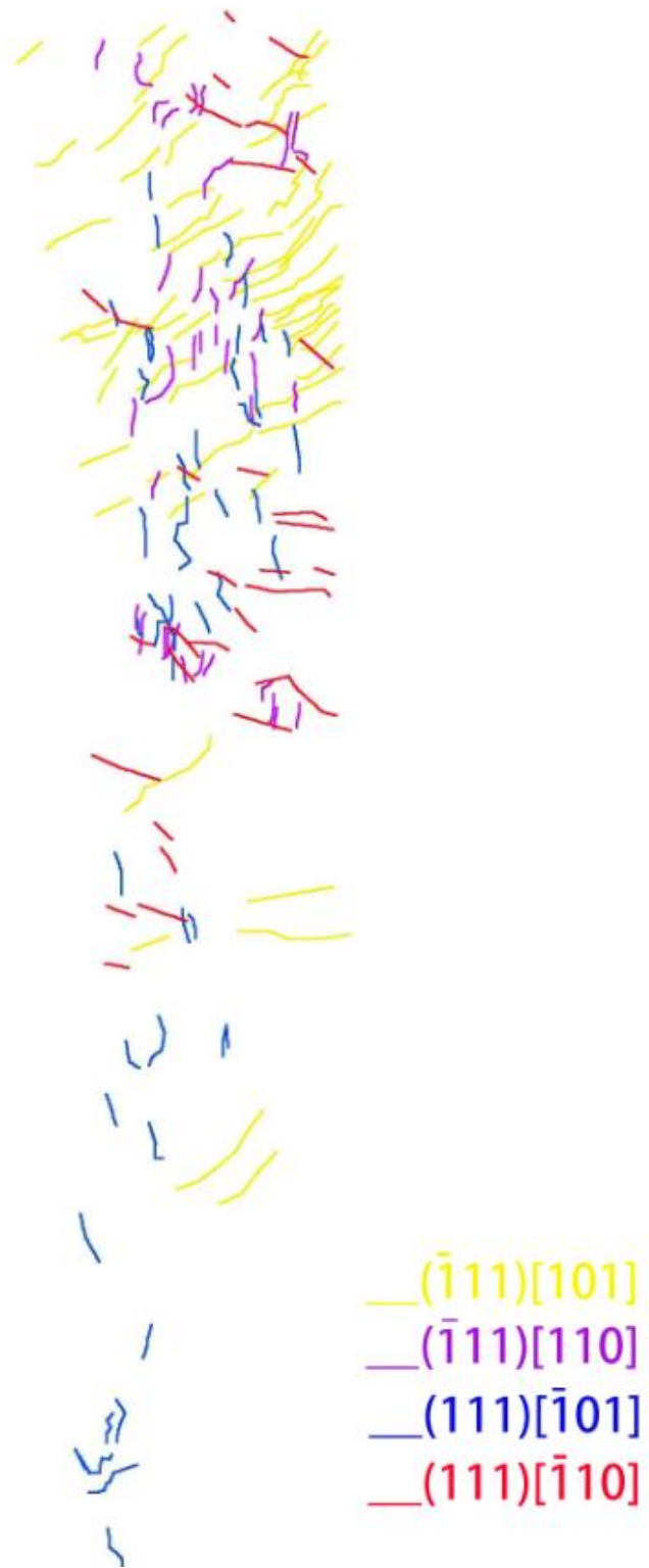
Figure 6-26 Colour-coding for the dislocations in the right hand 156 grain. The yellow and purple dislocations are traced from Figure 6-25 (c), the blue ones from (b) and the red ones from (a)
