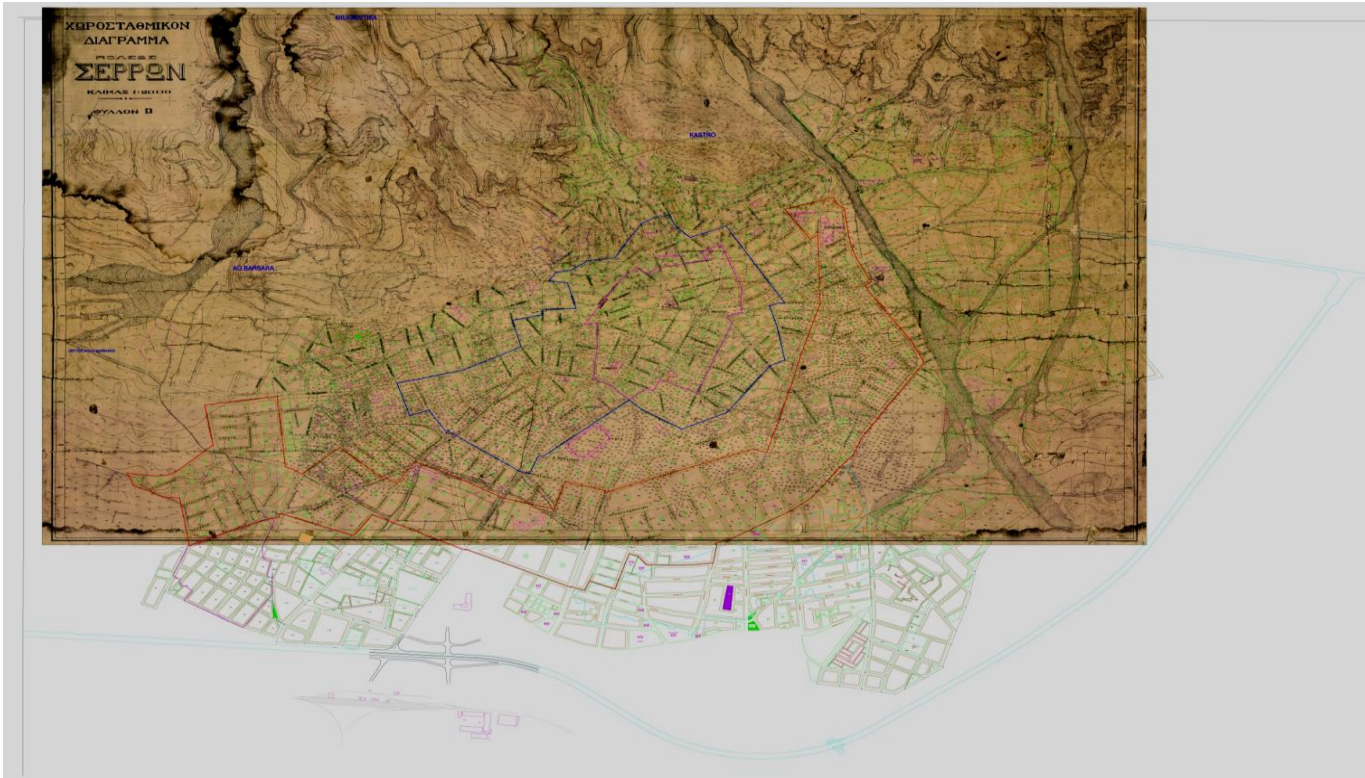
Map 6: The 1914 topographical survey of Siroz georefered using the 1994 street plan as a reference.
