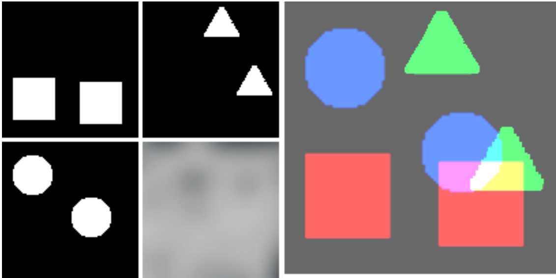
Figure 5.12: A simulated dataset consisting of simple shapes which consists of a set of overlapping geometric shapes with a fluctuating background. Each shape shares the same spectrum, mixed colours indicated overlaps and unique spectral regions.
