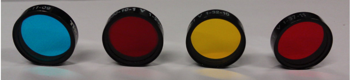
Figure 5.5: Photograph of a subset of the interference-based bandpass filters used in this work. From left to right the central wavelengths are 540, 700, 570, and 630nm.
