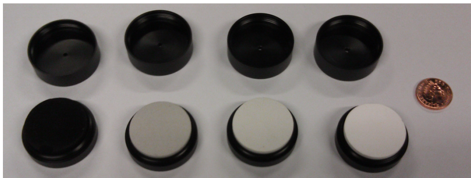
Figure A.5: Photograph of reflectance standards with a coin as a size reference, from left-to-right these are 2, 50, 75, and 99 percent reflective standards.
