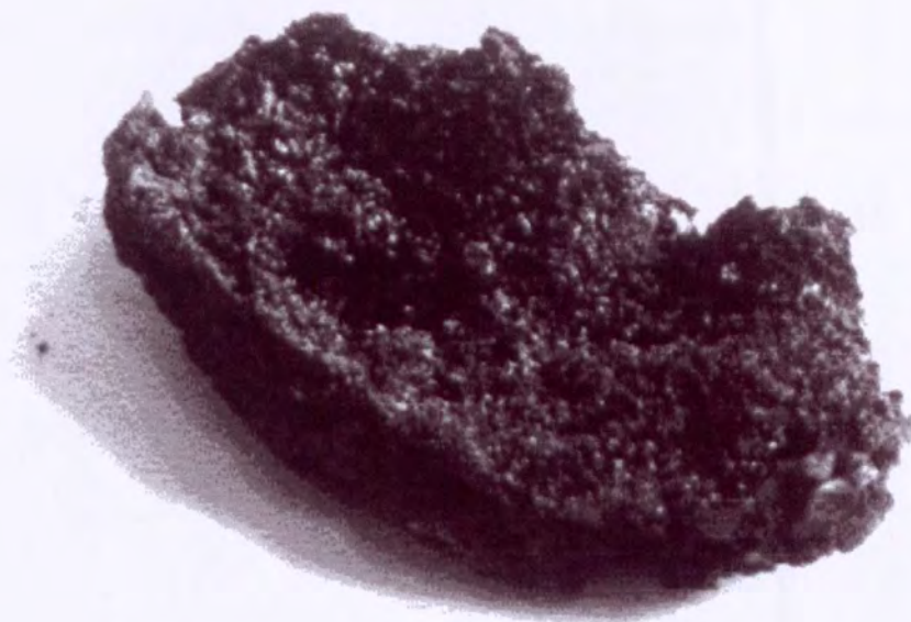
Figure 11.9 Coal pyrolysis after microwave heating
