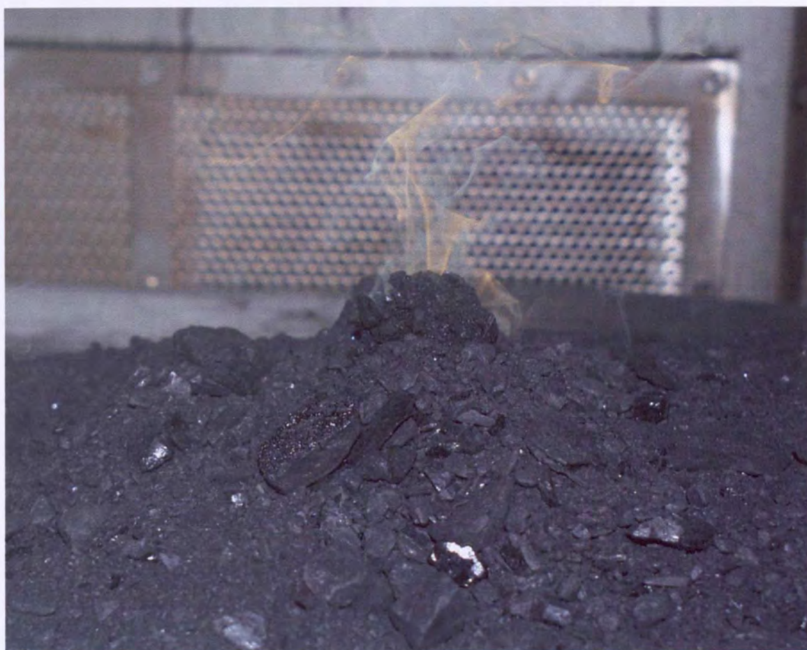
Figure 11.1 Sulphur release from coal prior to combustion within a microwave field
