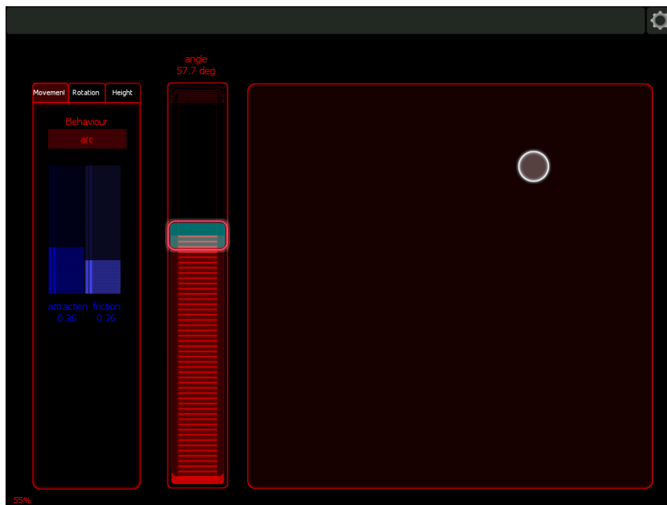
Fig. 7. Spatialisation interface for Lemur. The XY grid controls the x/y orientation of the centre point of the arc or swarm whilst the larger fader controls the width of the arc or attraction of the swarm particles.
