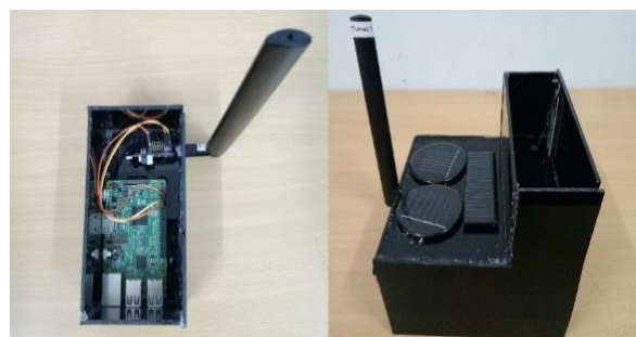
Figure 2. The master (right side) and slave (left side) nodes hardware
