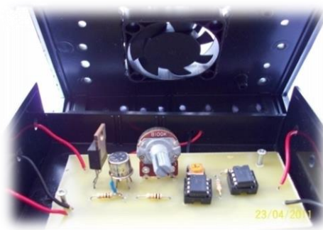
Figure 10. TGS2600 gas sensor measurement circuit
