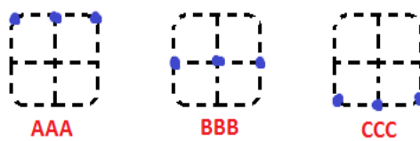
Figure 3. Matrix converter – zero vector modes
