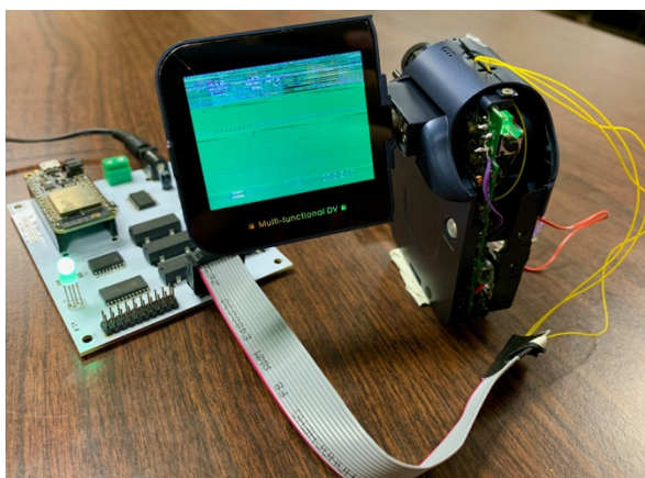
Figure 2: A circuit-bent camera connected to a Bendit board.
