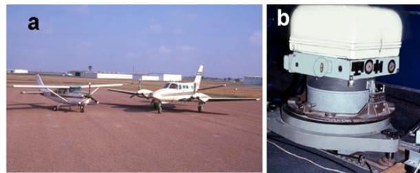
Fig. 4. Aircraft platforms and camera system used in aerial surveys of South Padre Island research sites: single-engine Cessna 206 and twin-engine Cessna 404 Titan (a) and Fairchild KA-2 camera with 12-in focal length lens (b) mounted in aircraft (courtesy of Agricultural Research Service, U. S. Department of Agriculture).
