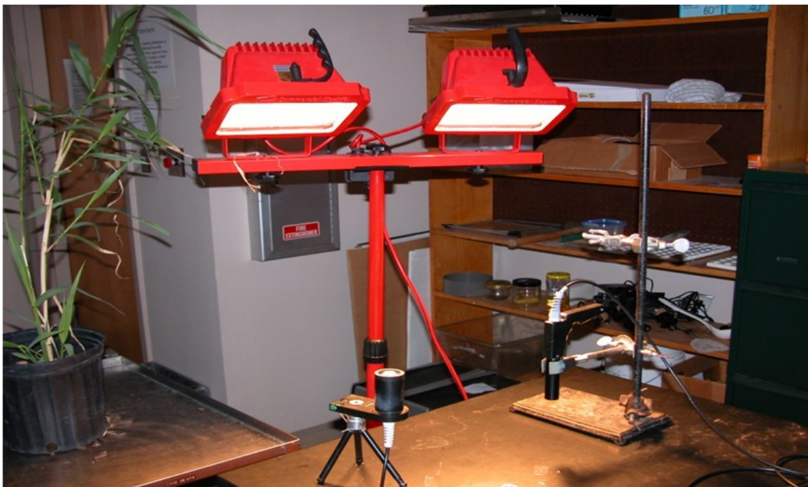
Fig. 1. Commercial Electric 500-w quartz halogen lamp used as an artificial lighting source for acquisition of spectroradiometer measurements and multispectral imagery under laboratory conditions (Summy et al. 2004).
