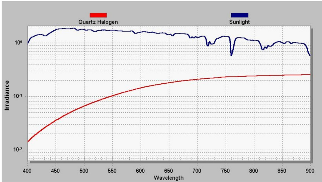
Fig. 5. Irradiance curves for sunlight and quartz halogen lamp used in the acquisition of spectroradiometer measurements under laboratory conditions. Data acquired at 11:00 am on 4 August 2011.
