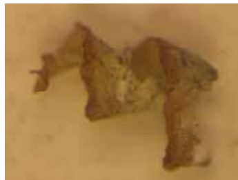
Figure 4.61: Continuous/spiral nylon peel ply chip
