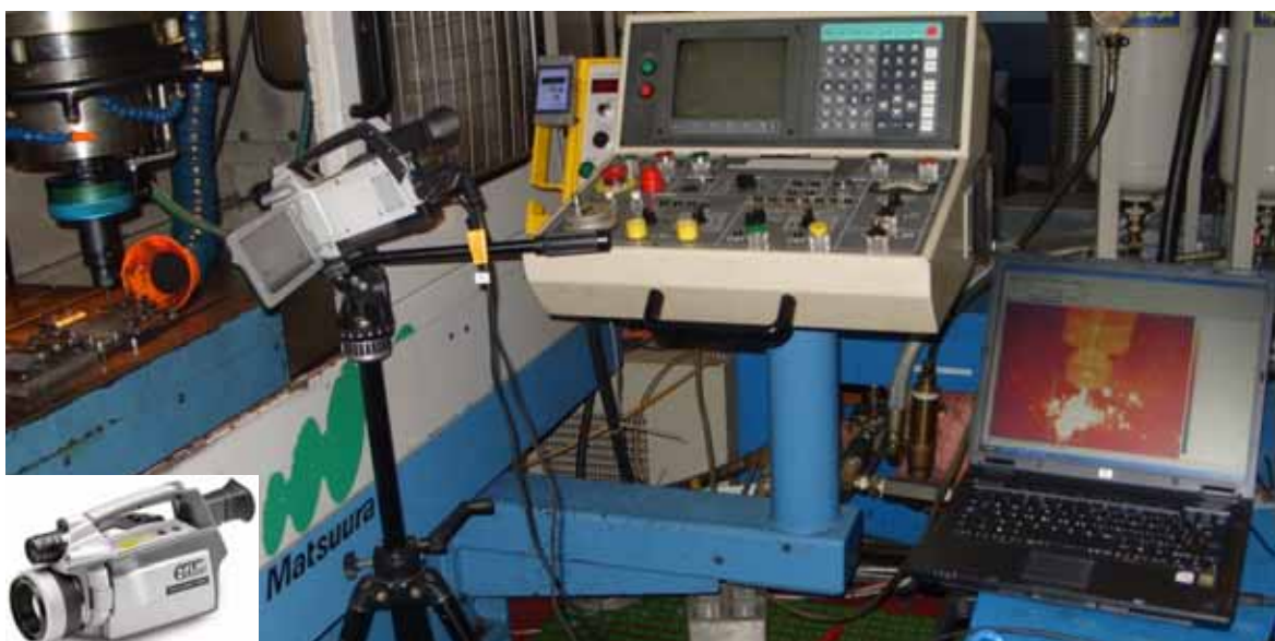
Figure E-1: Cutting temperature setup on Matsuura FX-5 using ThermaCAM which was loaned from EPSRC
