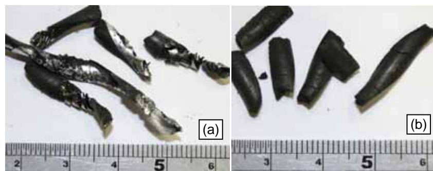
Figure 4.133: (a) CFRP particles fused with aluminium swarf and (b) CFRP chips formed according to contour of drill flutes
