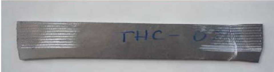
Figure 1: Geometry of the tested specimens 5182 H111 Aluminium alloy
