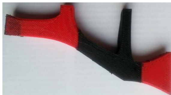
FIG 5 - Optimized structure printed with two different materials
