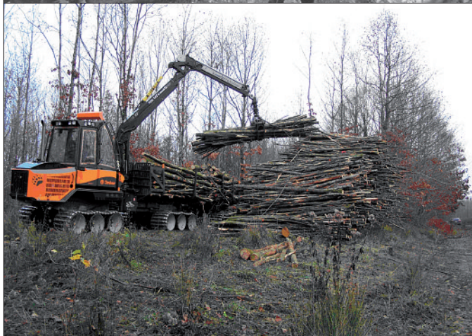
Photo 2. Hauling using a tracked forwarder in the state forest of Der (Haute-Marne) in 2010.
