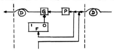
H. Platt explained the modifications he has made on the standard plug-in flip-flop to make it capable of driving as many as four gate tubes (an estimated capacitive load of 80  $\mu\mu f$ ), delaying .1  $\mu s$  after receiving a .1  $\mu s$  pulse before beginning to switch, and completing its switching in .3  $\mu s$ . Some seven circuit elements were changed in the flip-flop to obtain this performance.
