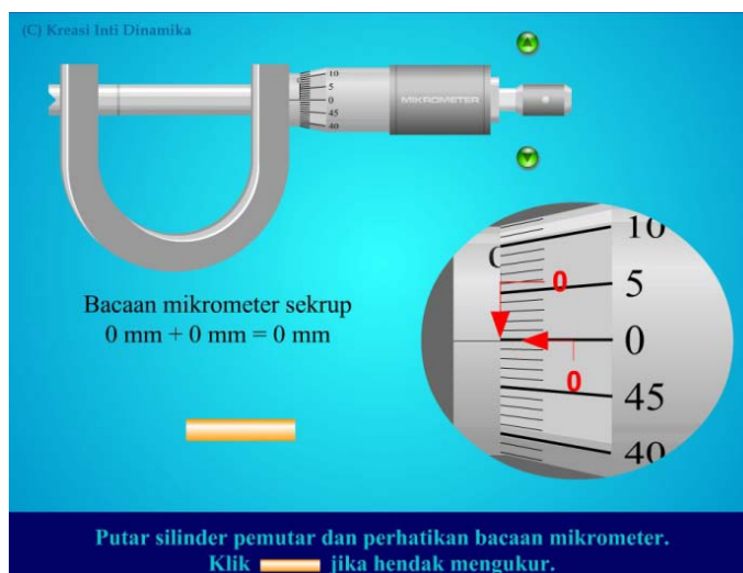
Gambar 45. Simulasi Outside Micrometer Tipe 2
