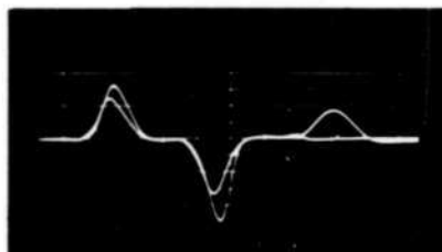
TOO LITTLE RESISTANCE IN COUPLING LOOP
